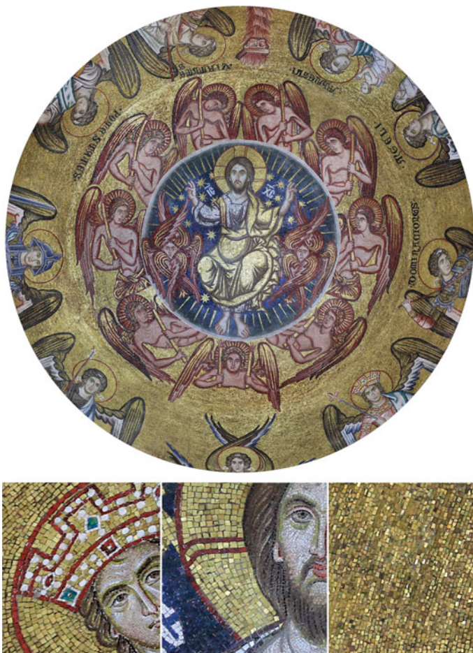
Fig. 5 The orthophoto of the dome of Baptistery, (top), with some details (bottom) where it is possible to see the smallest details of the golden tessera in the orthophoto (pixel size of 0.5 mm)
