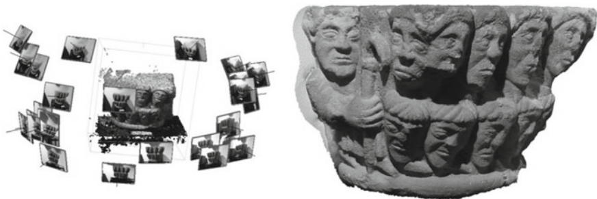
Fig. 4 On the left: camera poses used to reconstruct a Medieval capital. On the right: the final textured 3D model of the capital obtained from the projection of images
