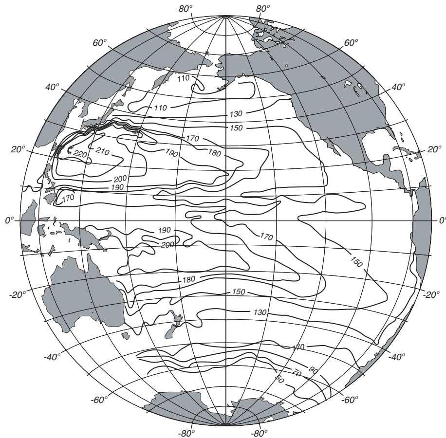
Figure 10.9. Mean geopotential anomaly relative to the 1,000 dbar surface in the Pacific based on 36,356 observations. Height of the anomaly is in geopotential centimeters. If the velocity at 1,000 dbar were zero, the map would be the surface topography of the Pacific. After Wyrtki (1979).
