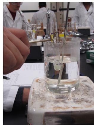
Figure 1.53: Boiling water bath.
