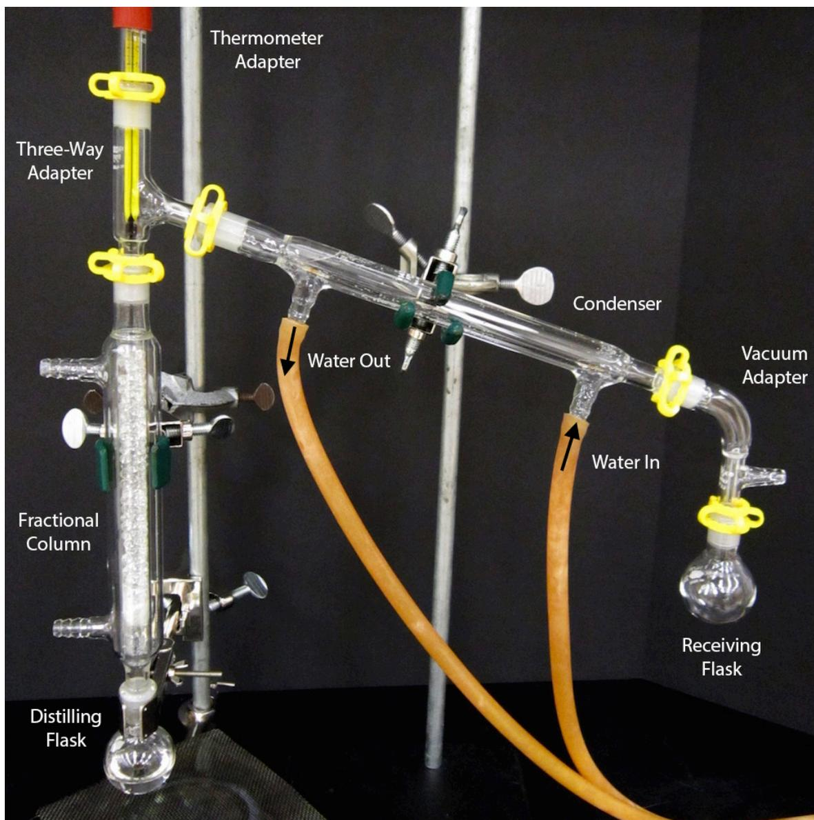
**Figure 5.46:** Fractional distillation setup.
