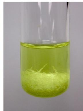
**Figure 3.19:** Yellow solid (benzil) in contact with cold ethanol.
