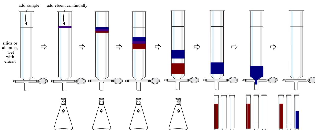
Figure 2.49: Schematic of column chromatography.
