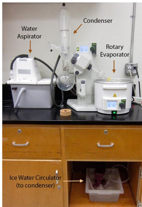
**Figure 5.65:** Rotary evaporator, water aspirator, and water circulator.
