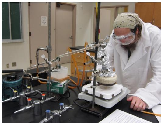
**Figure 5.54:** Student performs a vacuum distillation.
