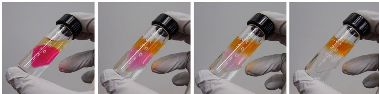
**Figure 4.35:** Progress of the extraction of methyl red from the acidic aqueous layer (bottom) into the organic layer (top). The inversions were done very slowly in order to see the extraction stepwise. With even gentle mixing, the methyl red (and thus color) extracts rapidly.
