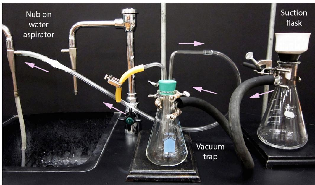
Figure 7.1: Suction filtration vacuum trap apparatus.
