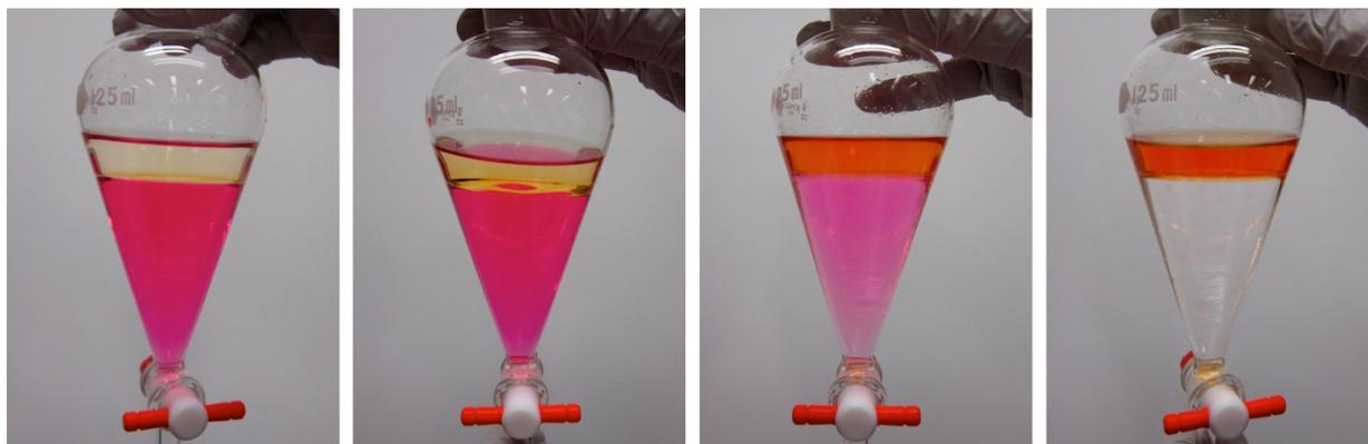
**Figure 4.20:** Progress of the extraction of methyl red (the colored compound) from the acidic aqueous layer (bottom) into the organic layer (top). The inversions were done very slowly in order to see the extraction stepwise. With even gentle mixing, the methyl red extracts rapidly.
