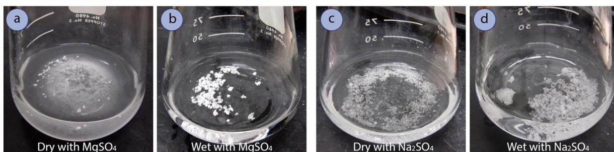
**Figure 4.52:** Drying ethyl acetate with anhydrous  $\text{MgSO}_4$  and  $\text{Na}_2\text{SO}_4$ : a) Dry  $\text{MgSO}_4$  (very fine particles), b) Wet  $\text{MgSO}_4$  (hydrate clumps), c) Dry  $\text{Na}_2\text{SO}_4$  (small particles), d) Wet  $\text{Na}_2\text{SO}_4$  (hydrate clumps).
