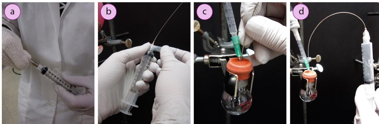
**Figure 1.33:** a) Screwing the needle onto the syringe head, b) Wrapping the joint with Parafilm, c) Inserting the needle into a flask filled with inert gas, d) Withdrawing inert gas in order to flushing the syringe.
