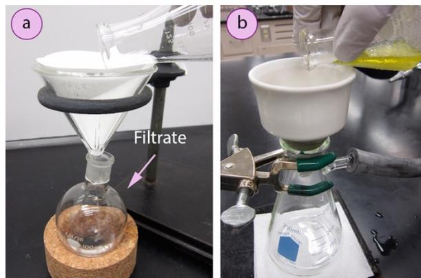
Figure 1.66: a) Gravity filtration, b) Suction filtration.
