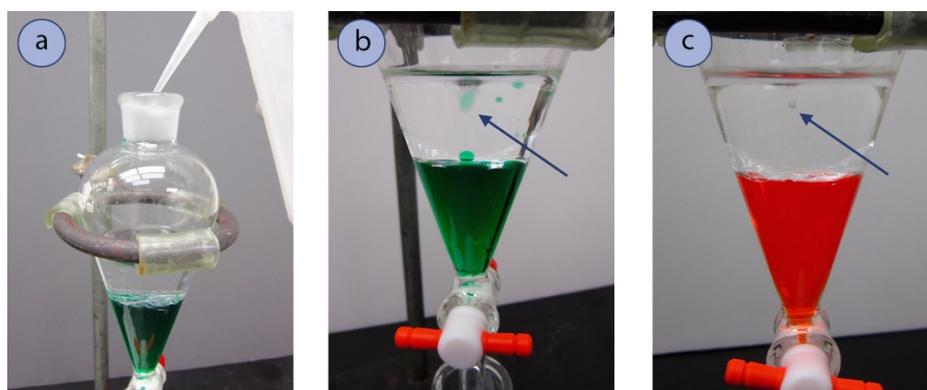
**Figure 4.9:** a) Adding water from a squirt bottle to determine which layer is aqueous, b) Water colored with green food dye is dropped into the funnel and falls to the bottom layer (aqueous), c) Water falling to the bottom layer, as indicated by the arrow.
