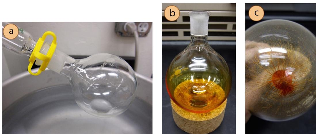
**Figure 5.71:** a) Residual liquid after evaporation, b) A sample after evaporation that left a film on the flask, c) The same sample that crystallized after allowing the flask to dry overnight.
