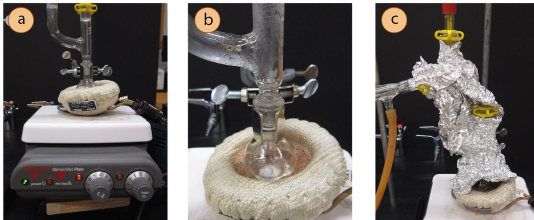
**Figure 5.52:** a) Stir plate with wood block to allow for lowering of the apparatus, b) Active distillation, c) Insulating the Claisen and three-way adapters with foil.
