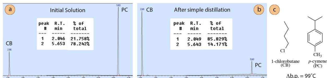
**Figure 5.10:** a) GC spectrum of a 75 mol% 1-chlorobutane and 25 mol% *p*-cymene mixture- note GC% need to be interpreted by a calibration curve. 1-chlorobutane is the peak at 2.1 min and *p*-cymene is the peak at 5.6 min, b) GC spectrum of the distillate from a simple distillation, c) Structures of 1-chlorobutane (CB) and *p*-cymene (PC).
