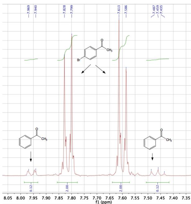
Figure 3.34: Partial 300 MHz <sup>1</sup>H NMR spectrum of the original mixture of 4-bromoacetophenone and acetophenone (two signals for the methyl groups are at 2.58 and 2.61 ppm). The integrations show a similar composition as the GC data.
