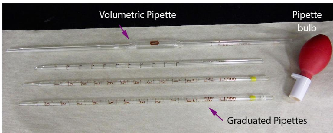
**Figure 1.22:** Volumetric and graduated pipettes.
