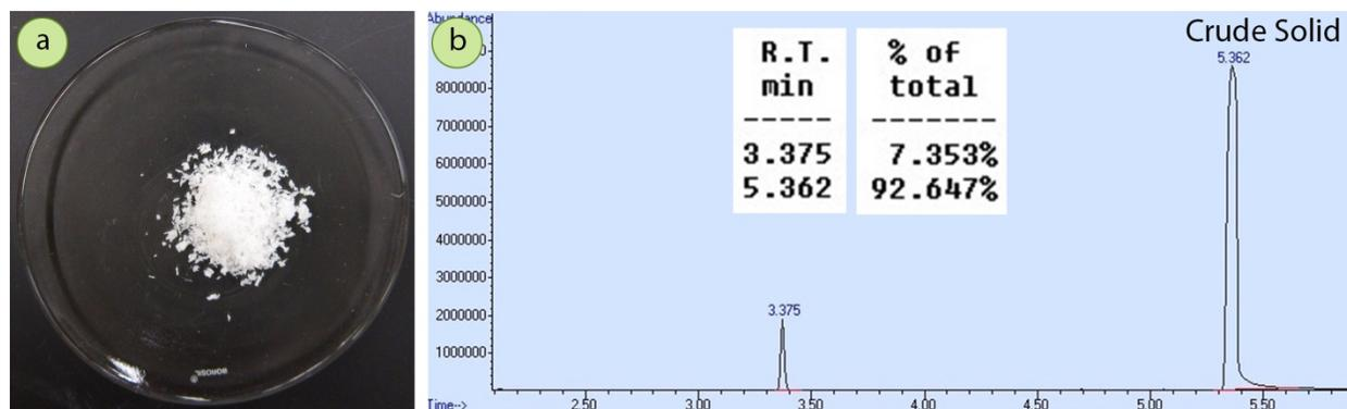
Figure 3.33: a) Initial solid mixture, b) GC spectrum of solid mixture.<sup>13</sup>
