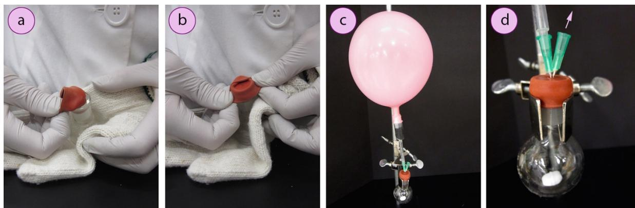
**Figure 1.32:** a+b) Alternative way to hold a hot flask and attach the rubber septum, c) Flushing a reaction flask with a gas balloon, d) Close-up of the “exit needle.”
