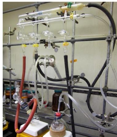
Figure 1.28: Gas manifold.
