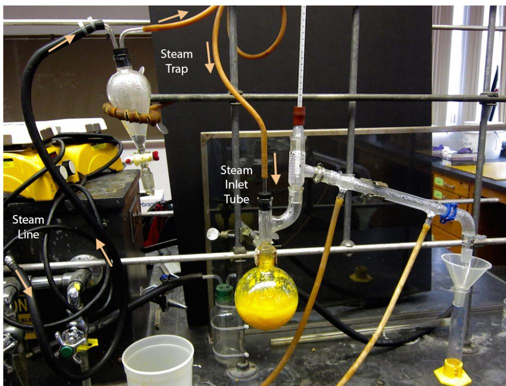
Figure 7.12: Steam distillation apparatus.
