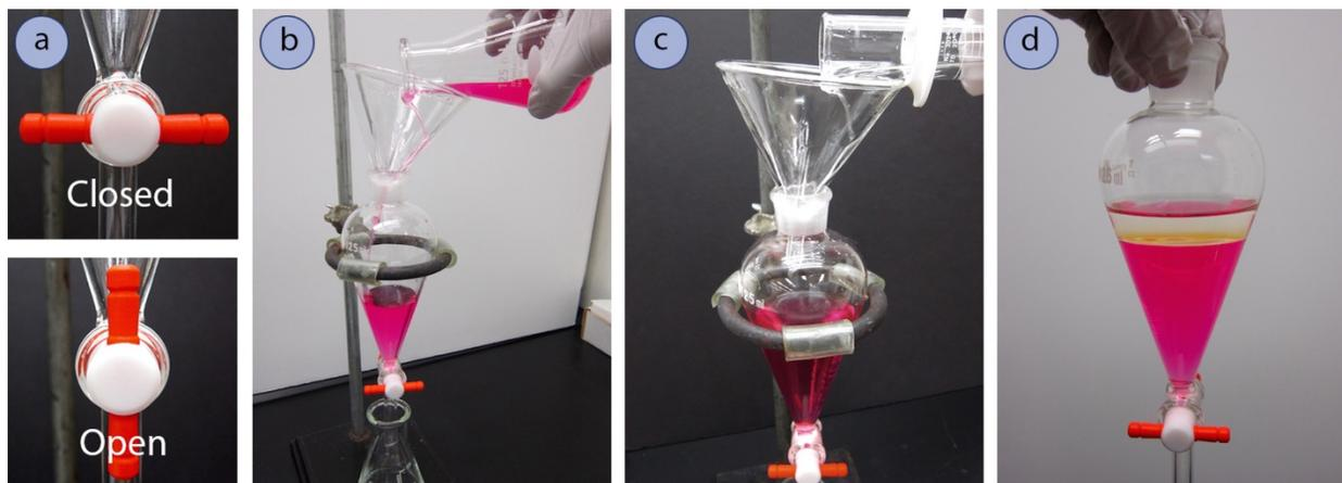
**Figure 4.24:** a) Closed and open stopcocks, b) Pouring in liquid with a funnel: notice the Erlenmeyer flask positioned below as a fail-safe, c) Pouring in the organic solvent, d) Separatory funnel before mixing.
