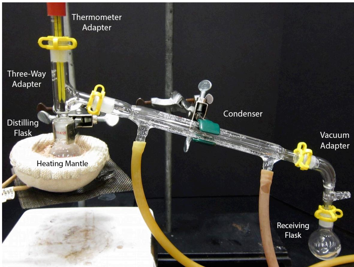
Figure 5.19: Simple distillation apparatus.
