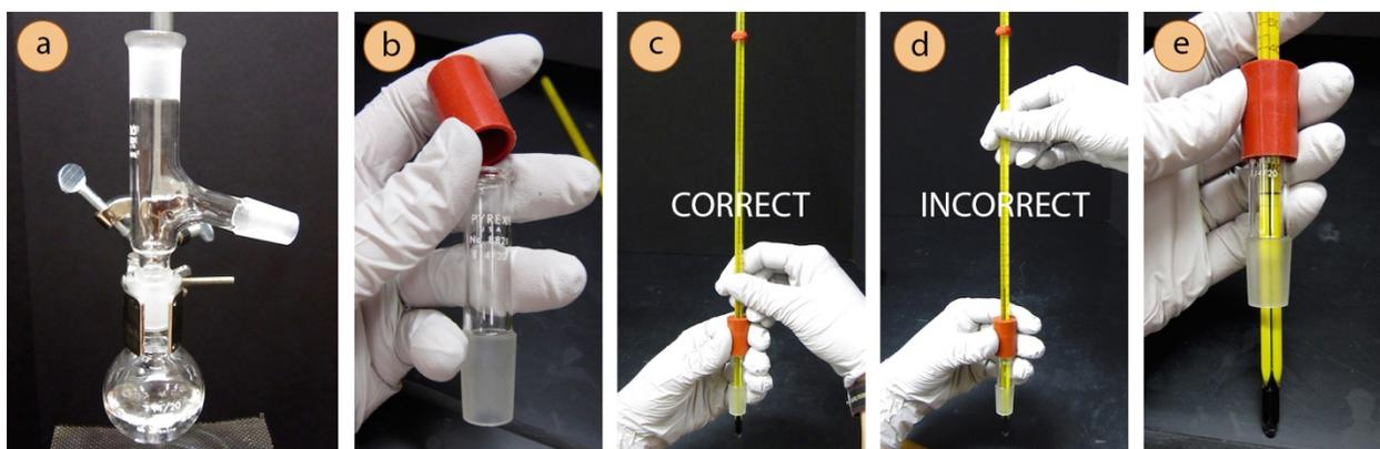
**Figure 5.22:** a) Flask and three-way adapter, b) Attachment of rubber fitting to thermometer adapter, c) Correct way to insert the thermometer, d) Incorrect way (thermometer will break), e) Assembled thermometer piece.
