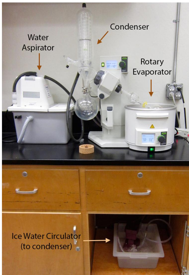
Figure 5.72: Rotary evaporation setup.
