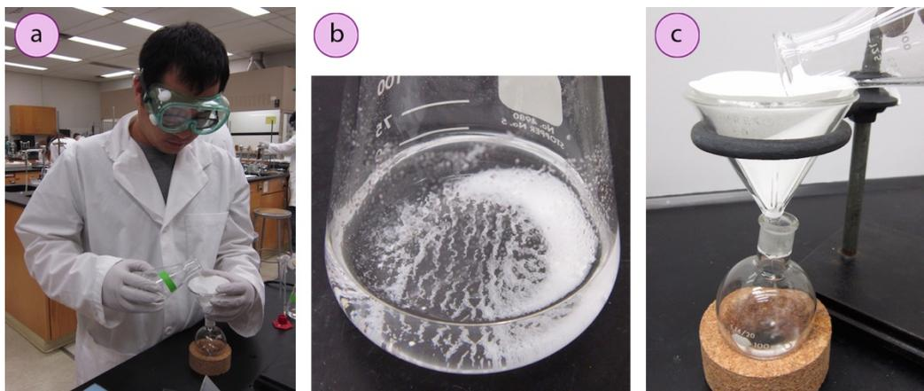
**Figure 1.68:** a) An organic solution dried with anhydrous magnesium sulfate, b) Gravity filtration of this solution.
