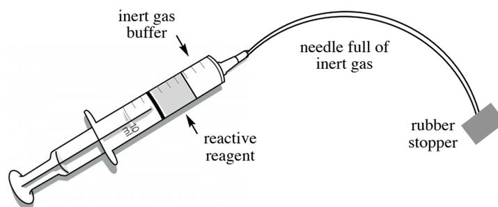
**Figure 1.36:** Syringe full of air-sensitive reagent ready for transport.
