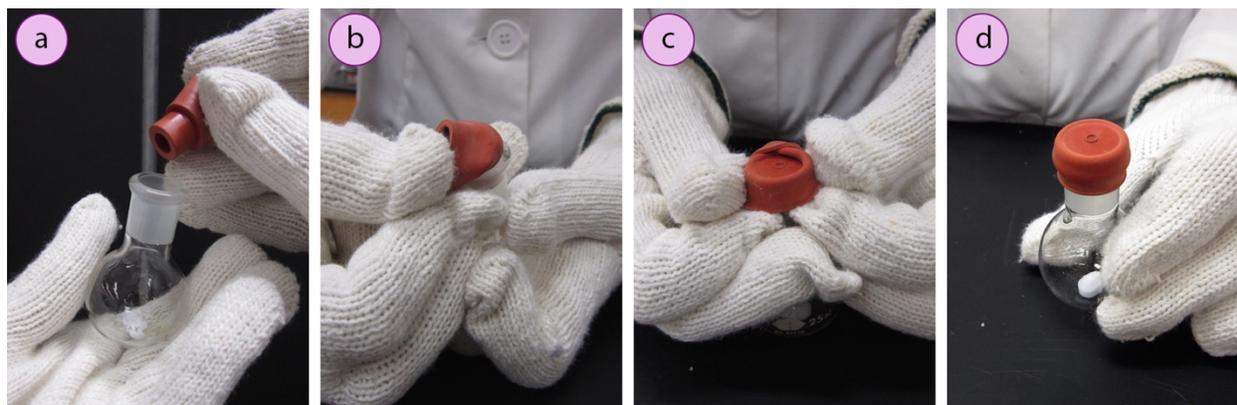
**Figure 1.31:** a) Inserting rubber septum into the joint of a hot flask, b-d) Folding septum flaps over the joint.
