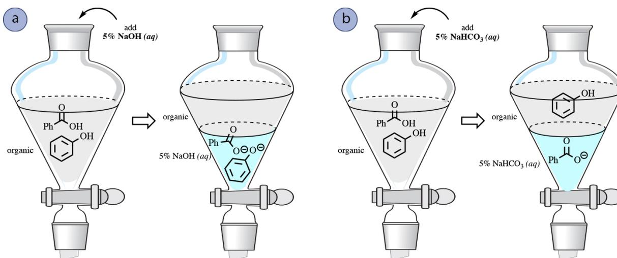
**Figure 4.58:** a) Extraction of both carboxylic acids and phenols into 5% NaOH (aq), b) Extraction of only carboxylic acids into 5% NaHCO<sub>3</sub> (aq).
