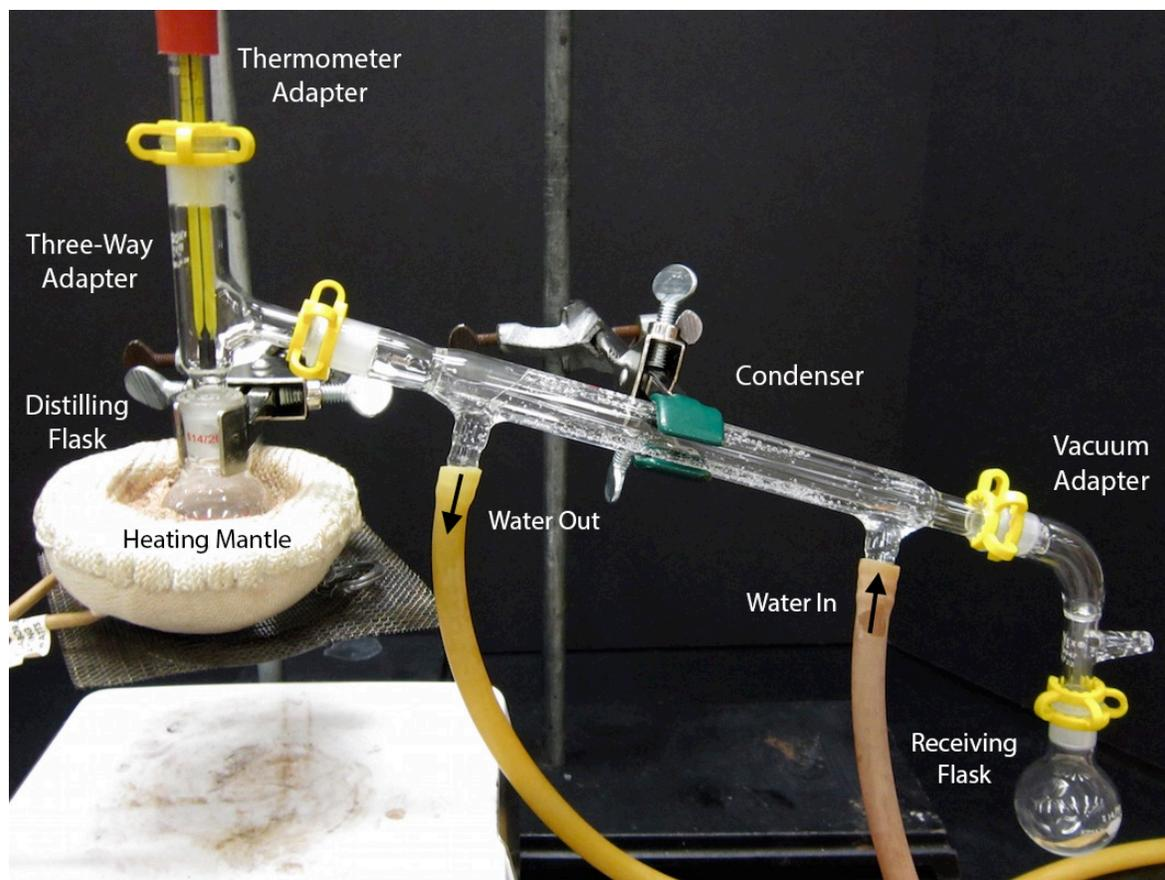
Figure 5.29: Simple distillation apparatus.
