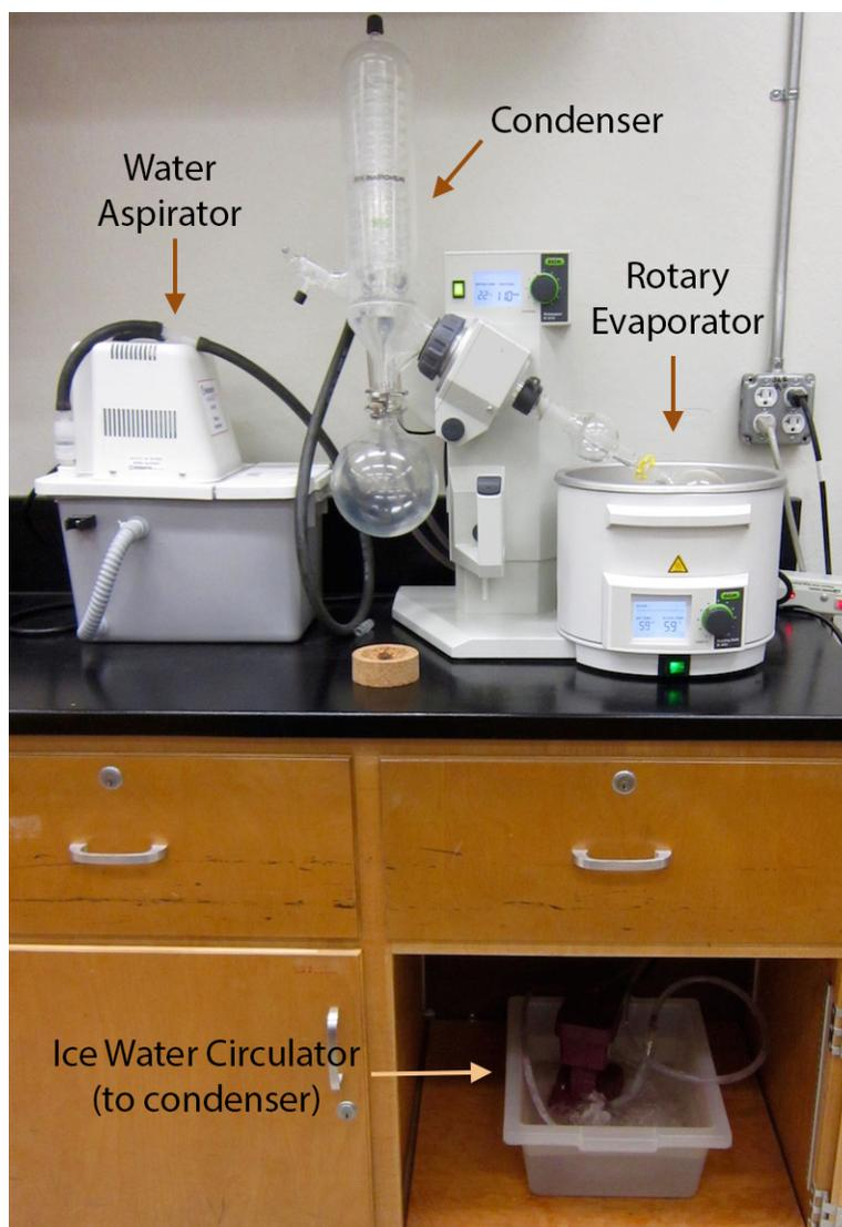
Figure 7.13: Rotary evaporation setup.
