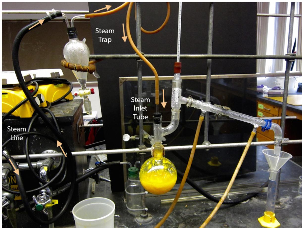
**Figure 5.59:** Steam distillation variation using a steam line from the building. Arrows show the direction of the steam.
