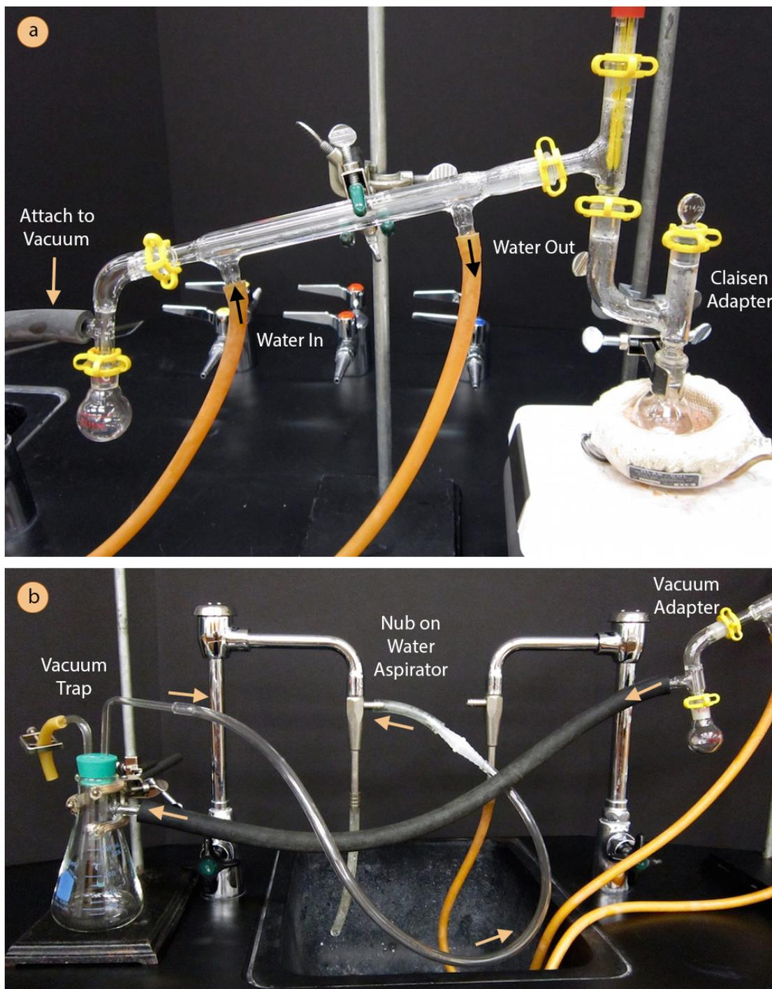
**Figure 5.50:** a) Vacuum distillation setup, b) Apparatus connected to a vacuum trap and water aspirator. Arrows show direction of suction.
