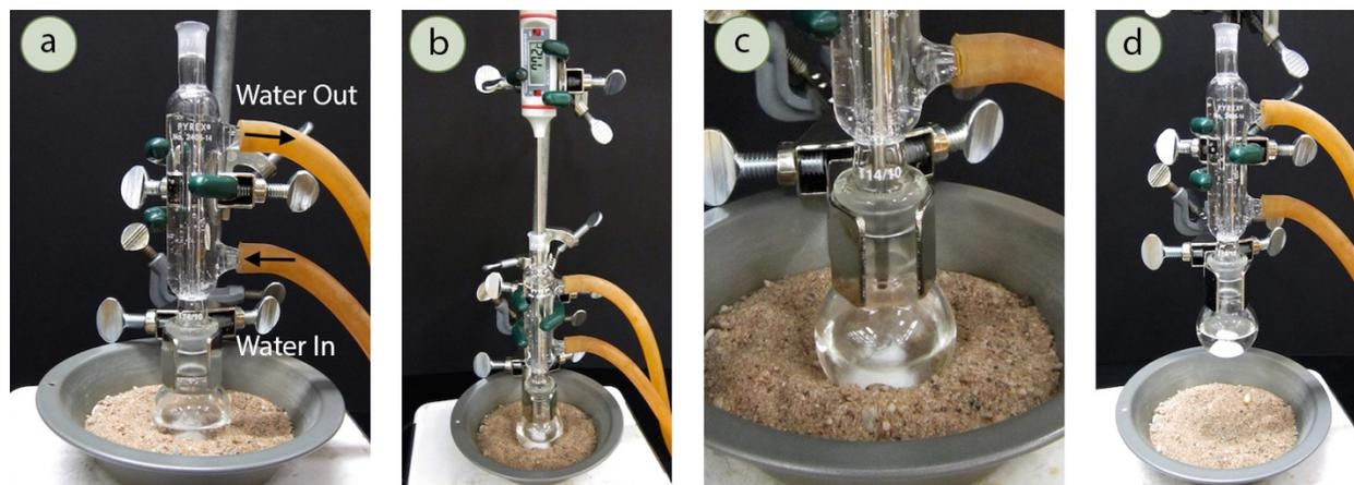
**Figure 6.20:** a) Reflux setup, b) Insertion of digital thermometer into condenser, c) Position of thermometer, d) Cooling the setup.
