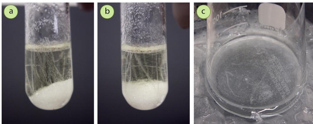
**Figure 3.46:** Lines of crystals seen in the initial stages of crystal growth, originating from where the glass was scratched: a+b) *N*-bromosuccinimide crystallizing from water, c) Acetanilide crystallizing from water.
