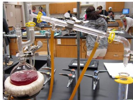
**Figure 5.2:** Distillation of fermented grape juice during a lab at Butte College.
