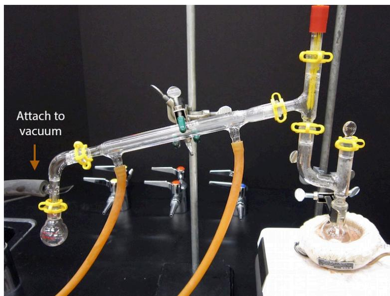
Figure 5.48: Vacuum distillation variation with a simple distillation.
