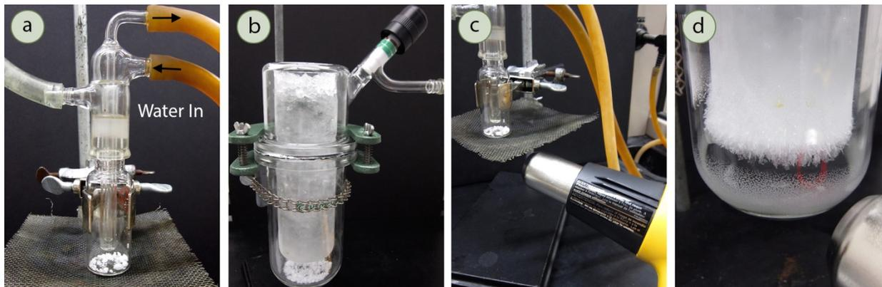
**Figure 6.34:** a) Small scale sublimation apparatus greased appropriately, b) Large scale sublimation apparatus with the cold finger filled with ice water, c) Heating the apparatus with a heat gun, d) Solid deposits on the outside of the glassware.
