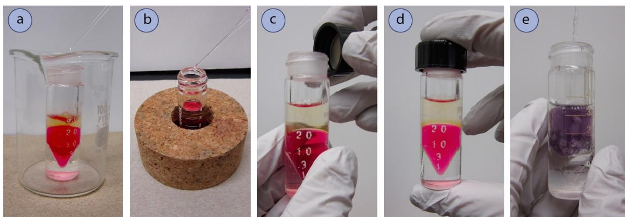
**Figure 4.36:** a) Adding solvent to the conical vial by pipette, and using a beaker to support the vial, b) Supporting the vial with a cork ring, c+d) Attaching the Teflon-lined cap to the vial, e) Manual mixing of layers (using a different system).
