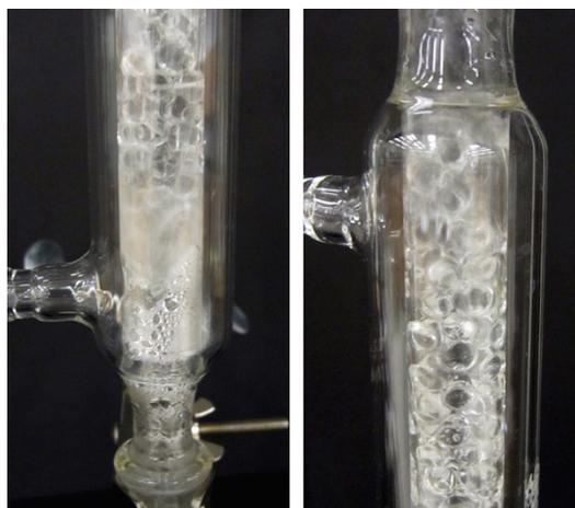
**Figure 5.45:** Flooding of a fractionating column.
