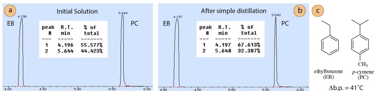
**Figure 5.12:** a) GC spectrum of a 75 mol% ethylbenzene and 25 mol% *p*-cymene mixture, note GC% need to be interpreted by a calibration curve. Ethylbenzene is the peak at 4.2 min and *p*-cymene is the peak at 5.6 min, b) GC spectrum of the distillate, c) Structures of ethylbenzene (EB) and *p*-cymene (PC).  $\Delta b.p. = 41\text{ }^{\circ}\text{C}$
