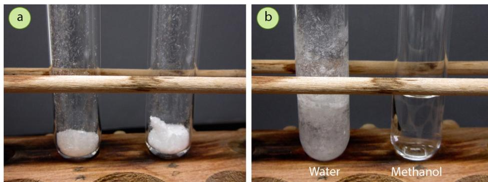
**Figure 3.14:** a) 100 mg of *trans*-cinnamic acid in each test tube, b) Left tube contains *trans*-cinnamic acid with water (insoluble) and right tube contains *trans*-cinnamic acid with methanol (soluble).
