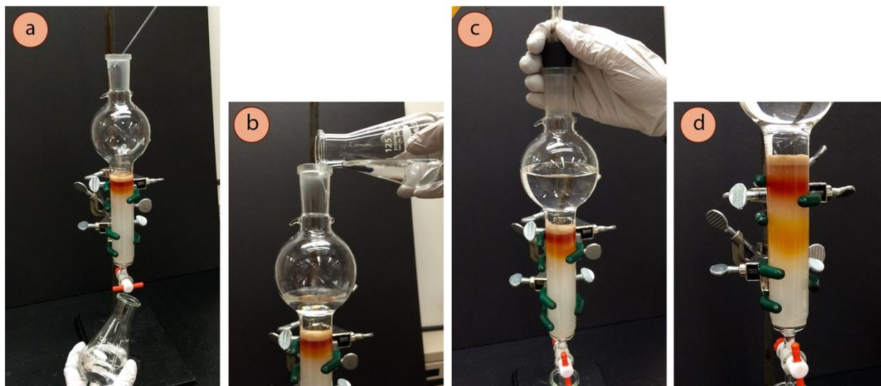
**Figure 2.57:** a+b) Filling the solvent reservoir, c+d) Eluting the column.
