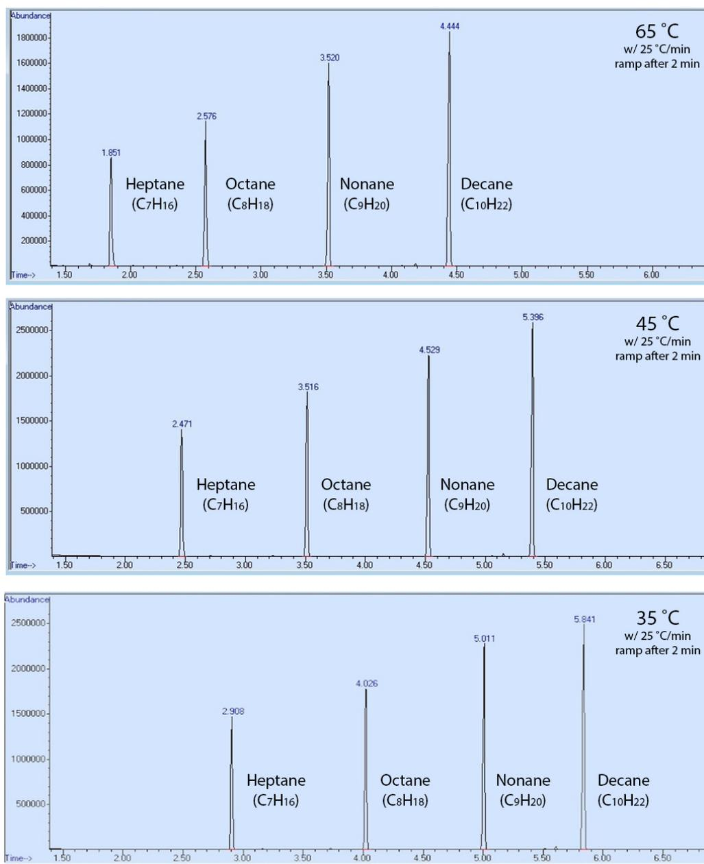
**Figure 2.90:** GC runs of a mixture containing heptane, octane, nonane, and decane at different oven temperatures. Each run was held at  $X$  °C ( $X = 65, 45, \text{ or } 35$ ) for 2 min, then ramped 25 °C /min.
