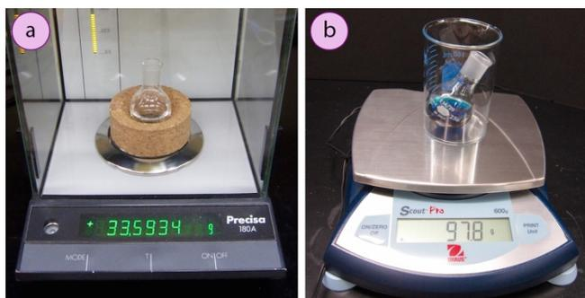
**Figure 1.18:** Round bottomed flasks supported by: a) Cork ring on an analytical balance, b) Beaker on a pan balance.
