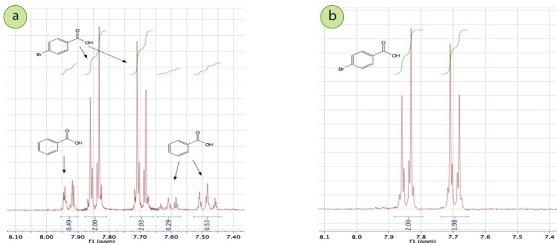
**Figure 3.6:** a) 300 MHz <sup>1</sup>H NMR spectrum of the crude mixture of benzoic acid and *p*-bromobenzoic acid (taken in DMSO-*d*<sub>6</sub>; carboxylic acid hydrogen is at 13.0 ppm and is not shown), b) <sup>1</sup>H NMR spectrum of solid after crystallization from ethanol, showing the sample is mostly *p*-bromobenzoic acid.
