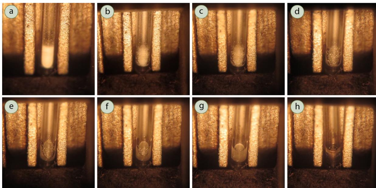
**Figure 6.2:** Time-lapse melting of benzoic acid: a) Well below the melting point, b) "Glistening" of the solid, c) First liquid droplet is seen (the temperature is recorded as the lower value of the melting range), d-g) Melting, h) Sample is completely melted (the temperature is recorded as the upper value of the melting range).
