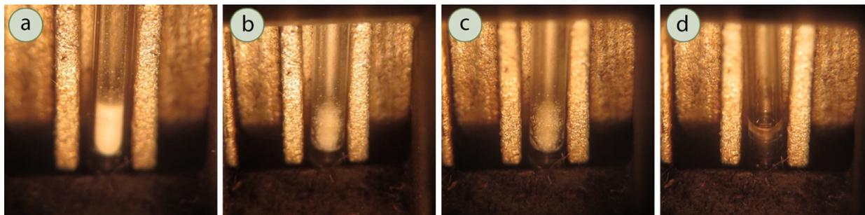
**Figure 6.13:** Melting of benzoic acid: a) Well below the melting point, b) Glistening, c) First liquid droplet seen, d) Sample is completely melted. Additional pictures for the melting of this sample can be seen in Figure 6.2.
