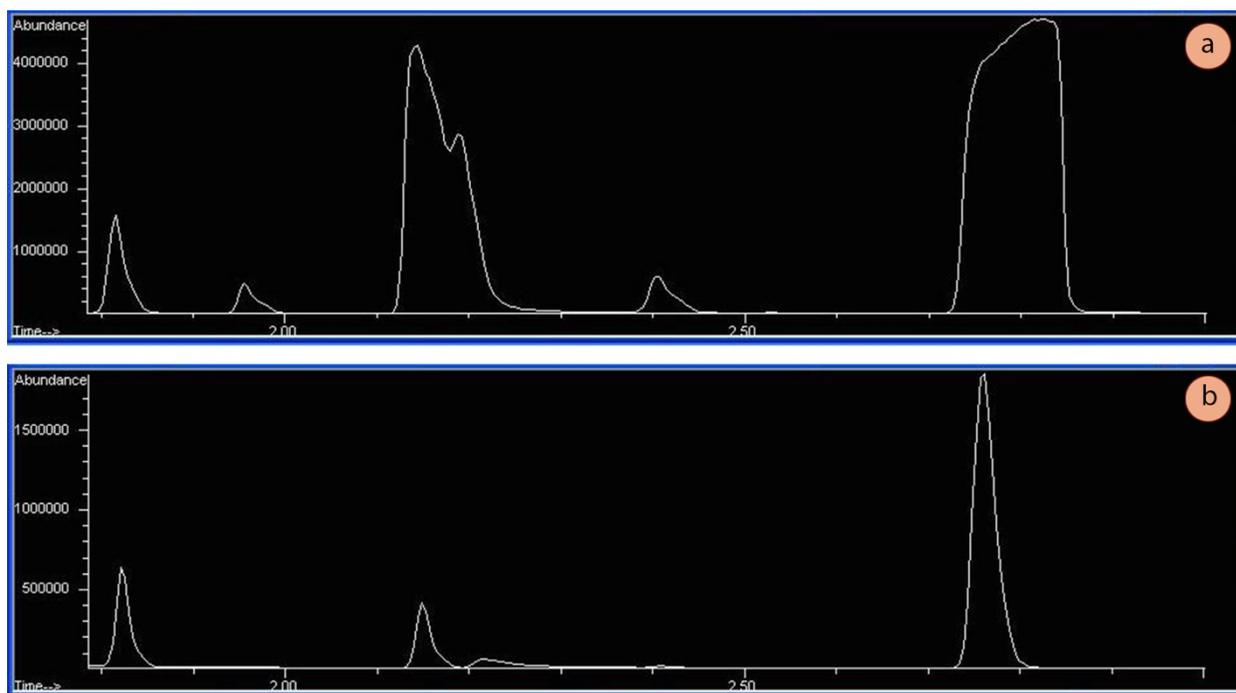
**Figure 2.87:** a) An overloaded sample with bad peak shape (note the y axis has abundances around 4.5 million), b) The same sample diluted appropriately (abundances around 2 million). A too dilute sample will have abundances less than 100,000 (MS detector).
