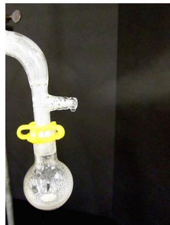
**Figure 5.33:** Vapor escaping from vacuum adapter.
