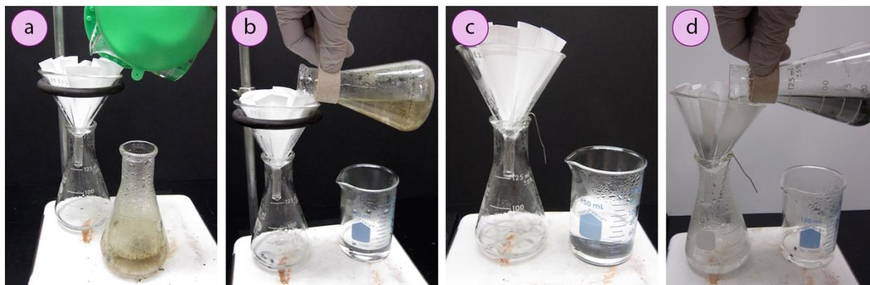
**Figure 1.81:** a) Pouring solvent through the funnel to get funnel hot (note: hotplate is used in this situation as the solvent is water), b) Filtering a solution containing insoluble impurities, c+d) Variations using a paper clip instead of a ring clamp to hold the funnel.
