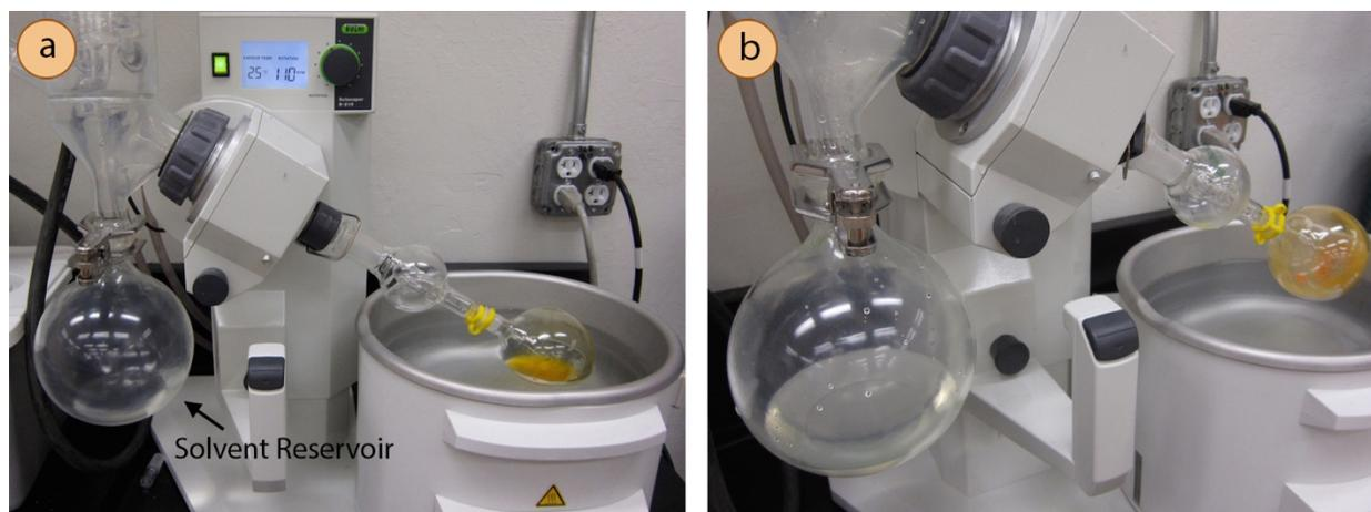
**Figure 5.70:** a) Evaporating a solution (with arrow pointing to the solvent reservoir), b) Formation of solid in the flask.
