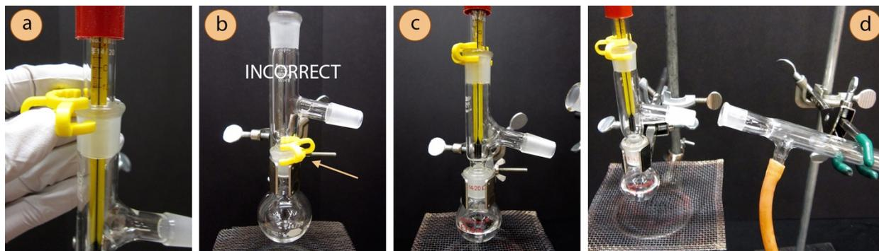
**Figure 5.23:** a) Connecting a plastic clip to secure a joint, b) Incorrect clamping: a plastic clip should not be used to connect the distilling flask to the three-way adapter (as indicated with the arrow), c) Correct positioning of thermometer in the three-way adapter, d) Preparing the condenser.
