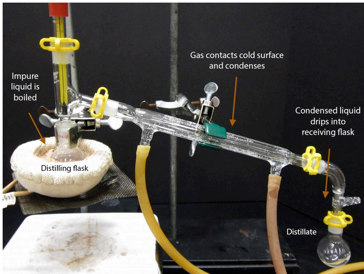
**Figure 5.1:** Basic process of a distillation (simple).
