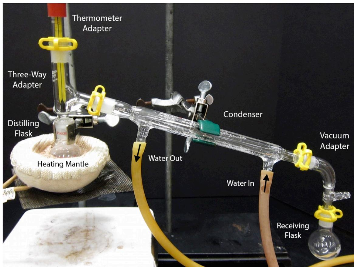
Figure 7.9: Simple distillation apparatus.
