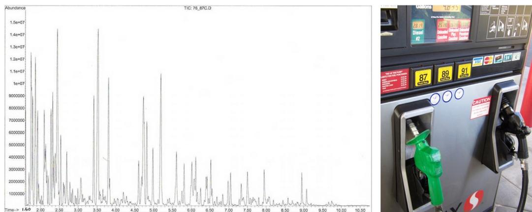
**Figure 2.76:** GC spectrum of 87 octane gasoline.
