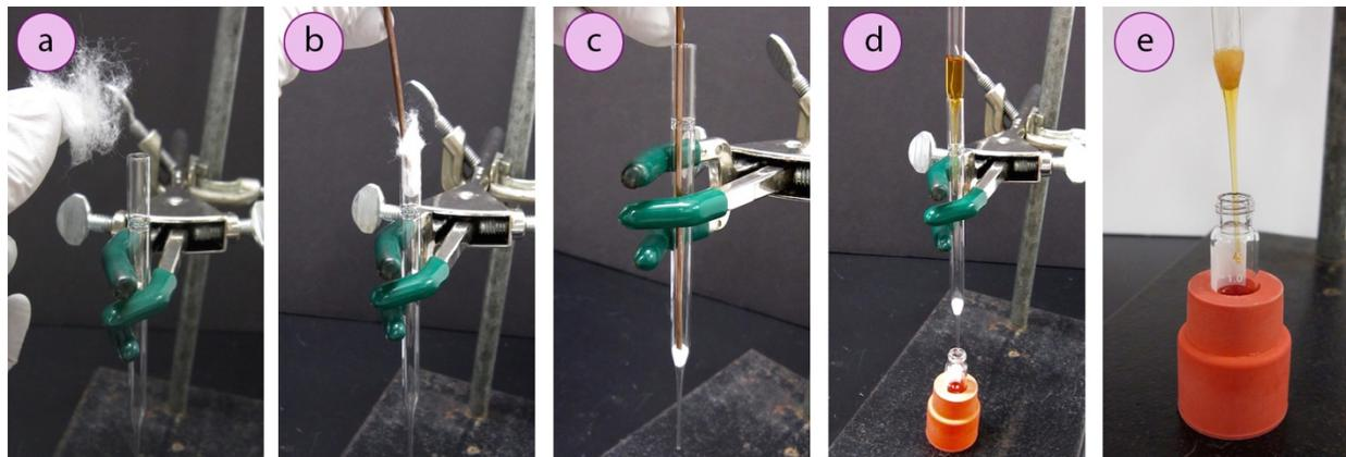
**Figure 1.89:** Creating and using a filter pipette: a) Piece of cotton, b+c) shoving cotton to the bottom of the pipette, d) Filtering a mixture into a GC vial, e) GC vial held with an upside down large septum.
