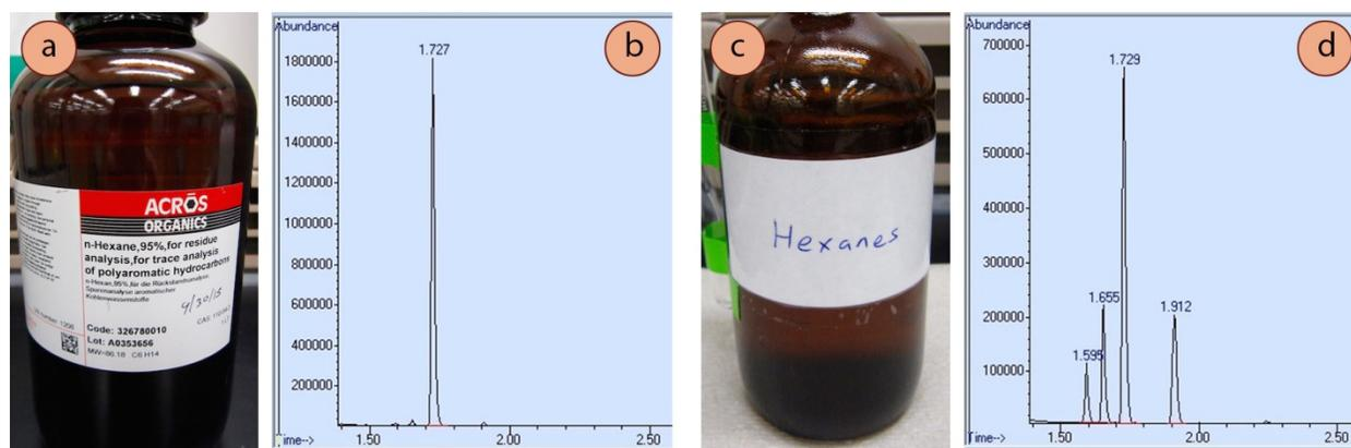
**Figure 2.77:** a) Bottle of *n*-hexane, b) GC spectrum of *n*-hexane, c) Bottle of “hexanes,” d) GC spectrum of “hexanes.” The compounds present in hexanes are: 2-methylpentane, 3-methylpentane, *n*-hexane and methylcyclopentane (in order of elution).<sup>13</sup>
