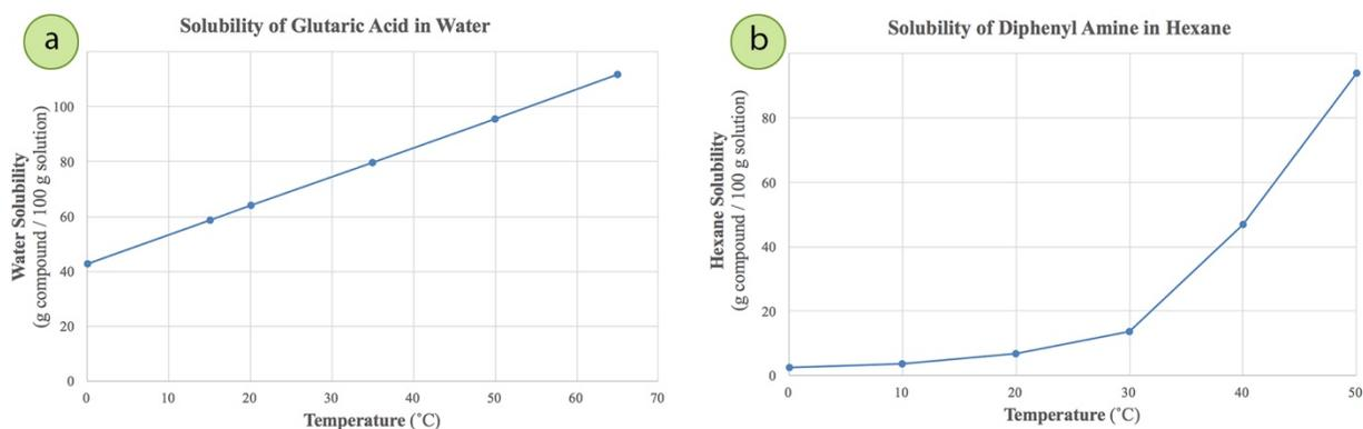
**Figure 3.8:** Solubility versus temperature data for glutaric acid in water (left) and diphenyl amine in hexane (right).<sup>3</sup> In both sets, solubility increases with temperature. Note that glutaric acid could not be crystallized from water, as it is highly soluble even at cold temperatures.
