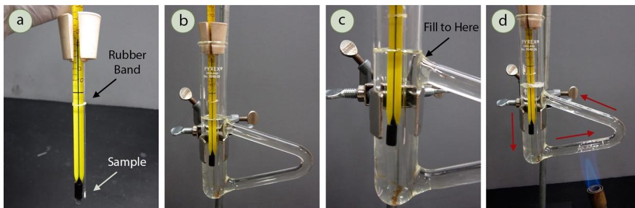
**Figure 6.15:** a) Capillary sample attached to a thermometer with a small rubber band, b) Placement of the sample in the Thiele tube, c) Correct location of the sample, with an arrow indicating the minimal height of mineral oil in the tube, d) Heating the Thiele tube with a burner, and arrows showing the oil current.
