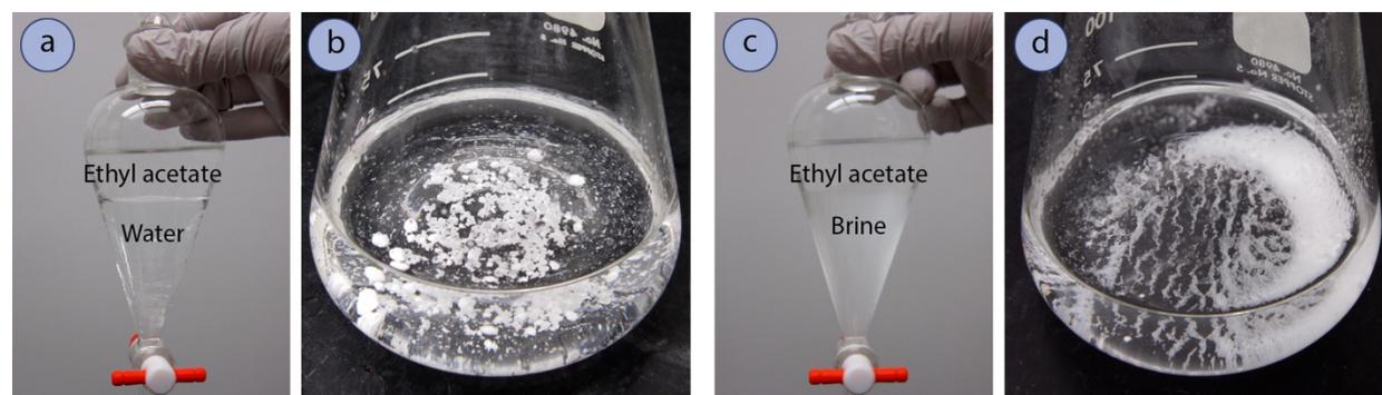
Figure 4.44: a) Ethyl acetate and water layers shaken together, b) Appearance of the ethyl acetate layer upon addition of anhydrous MgSO<sub>4</sub>, c) Ethyl acetate and brine layers shaken together, d) Appearance of the ethyl acetate layer with anhydrous MgSO<sub>4</sub>.
