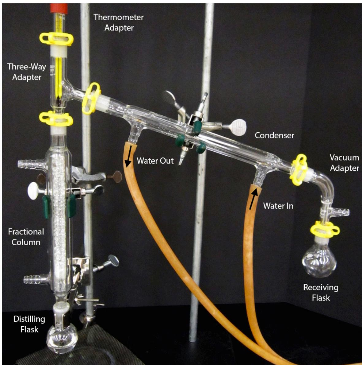
Figure 7.10: Fractional distillation apparatus.
