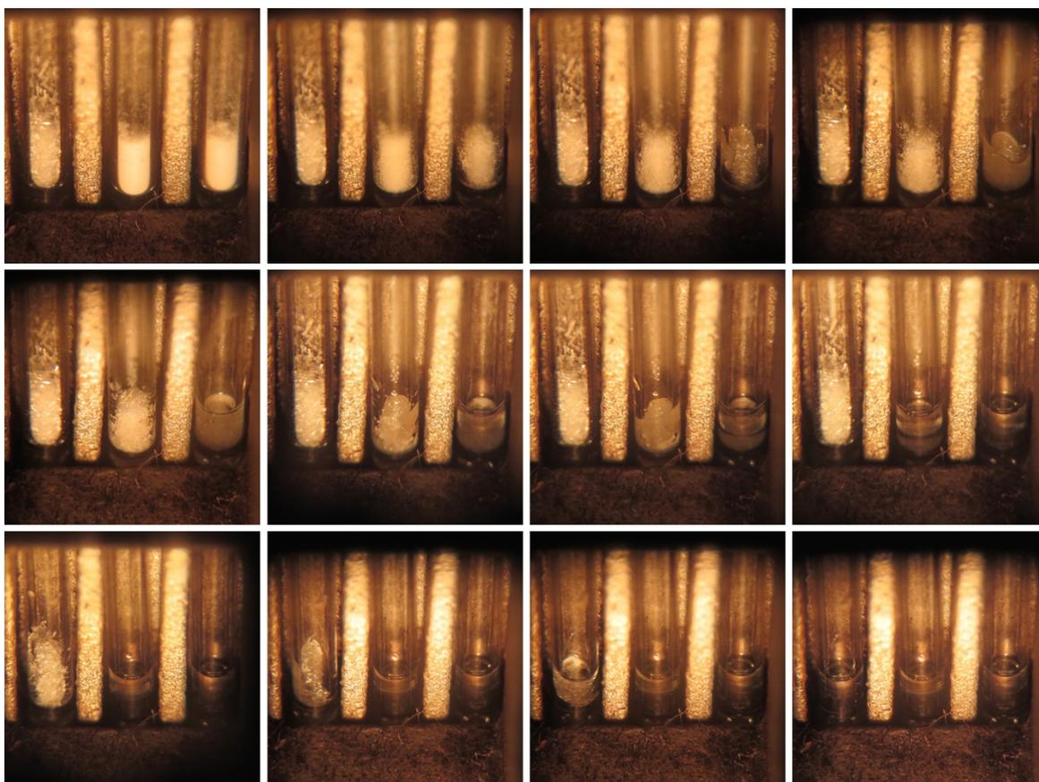
**Figure 6.5:** Time-lapse melting of three samples side by side in a melting point apparatus. Pure benzoic acid (left), benzoic acid with 10 mol% acetanilide (middle), benzoic acid with 20 mol% acetanilide (right).
