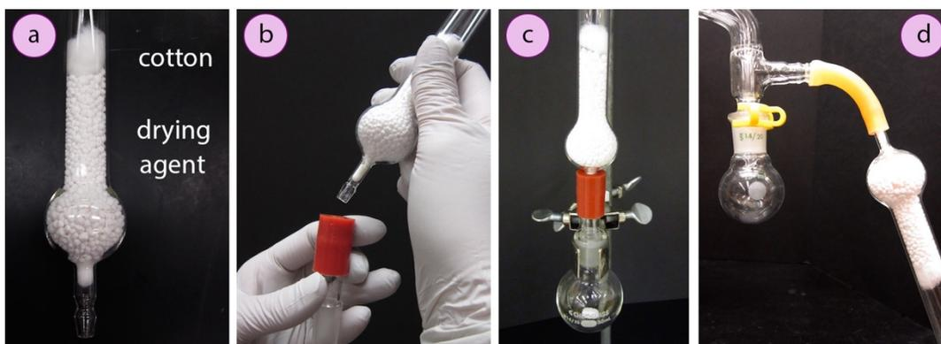
**Figure 1.13:** a) Drying tube with anhydrous  $\text{CaCl}_2$ , b) Inserting drying tube into a thermometer adapter, c) Drying tube attached to a round bottomed flask, d) distillation apparatus.
