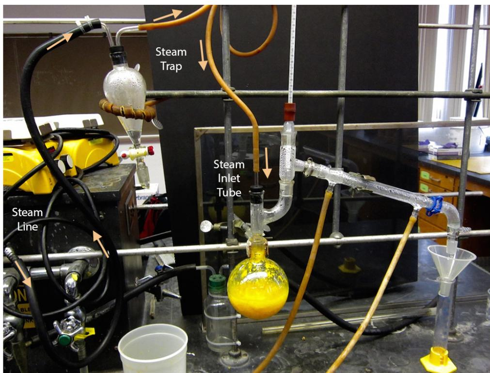
Figure 5.64: Steam distillation apparatus.
