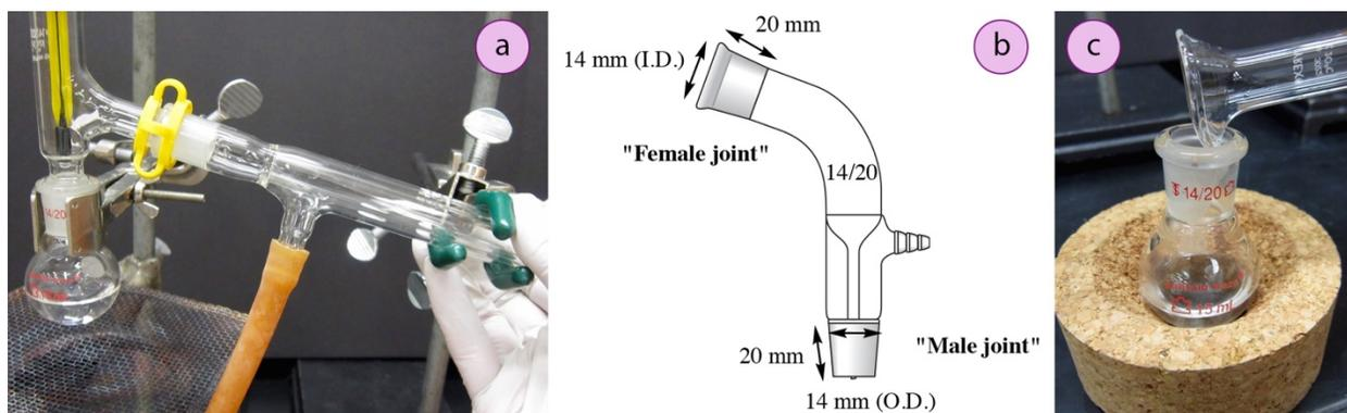
**Figure 1.1:** a) Connections of ground glass joints, b) Ground glass joint measurements (for a 14/20 piece of glassware), c) Pouring liquid into a flask.
