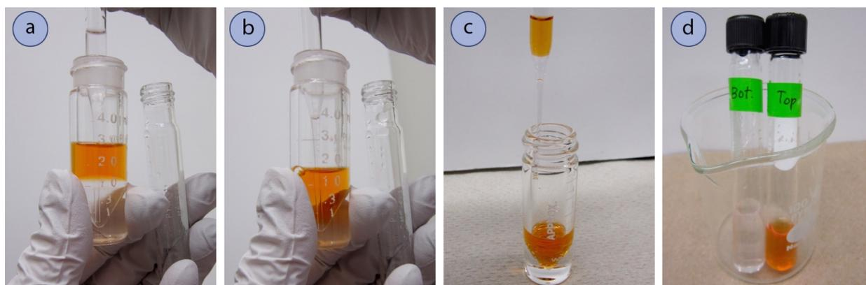
**Figure 4.37:** a+b) Withdrawal of the bottom layer, with pipette into the tip of the vial, c) Removal of a residual drop of the bottom layer by allowing the layers to separate inside a Pasteur pipette, d) Separated layers.
