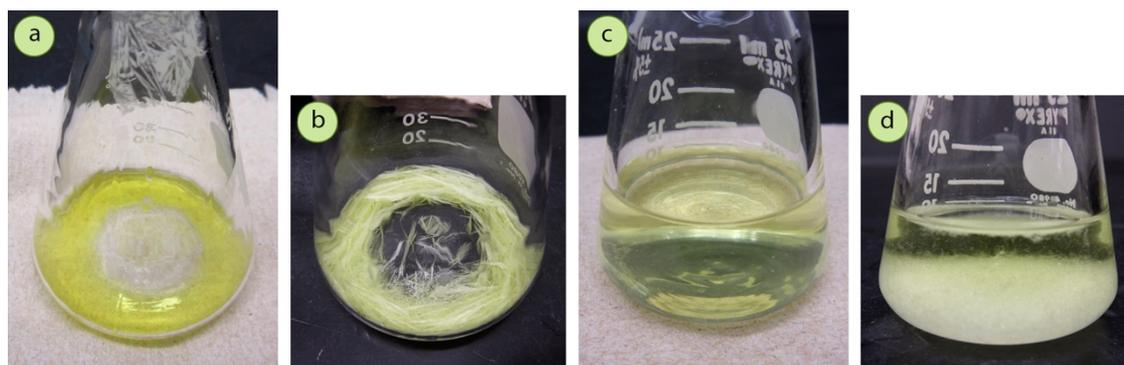
**Figure 3.44:** a) The flask is too large for the sample, and the solvent is too shallow, b) After crystallization the solvent is completely absorbed (or evaporated), c) The flask is the correct size for the amount of sample, d) The solvent is an appropriate height in the flask.
