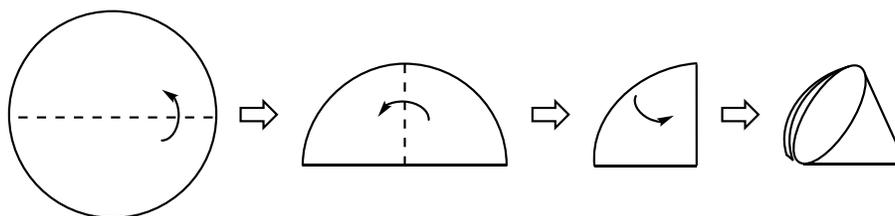
**Figure 1.69:** Creating a quadrant-folded filter paper. The dotted lines represent locations to crease and fold the filter paper. The arrows show the direction of folding.
