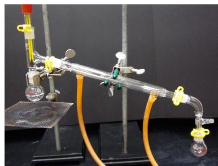
Figure 6.19: Simple distillation.
