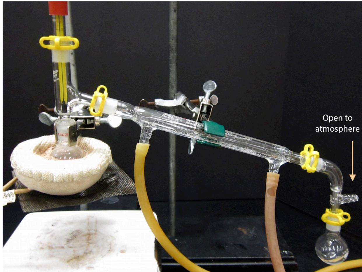
Figure 5.25: Completed simple distillation setup.
