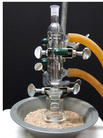
Figure 1.58: Reflux apparatus.
