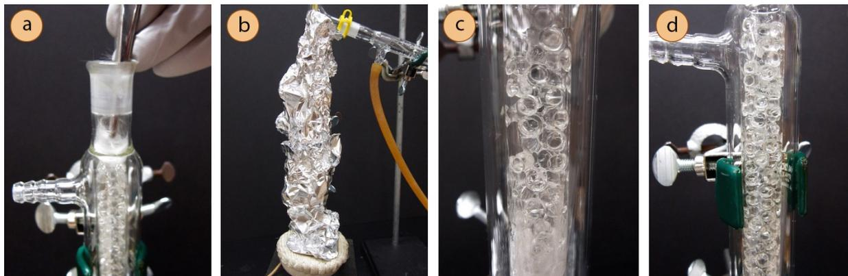
**Figure 5.44:** a) Removal of glass wool plug on a beaded fractionating column, b) Insulating the column, c+d) Condensation on the beads of a fractionating column.
