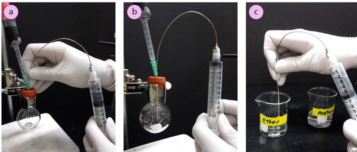
**Figure 1.37:** a) Inserting the syringe into the reagent flask, b) Delivering the liquid, c) Rinsing the needle and syringe.
