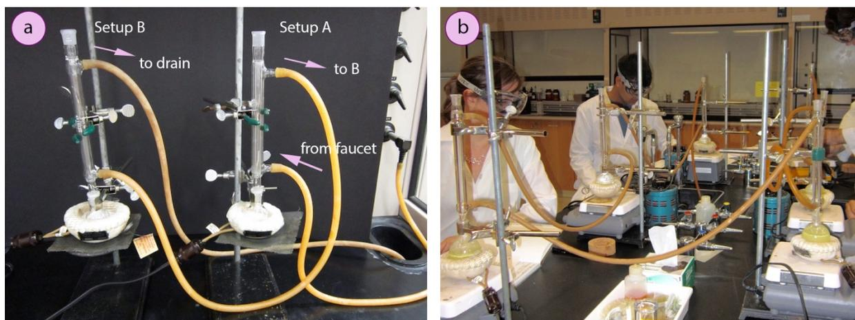
**Figure 1.62:** Connecting reflux condensers in series.
