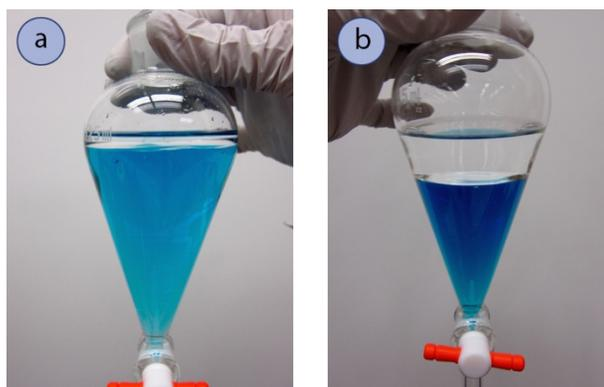
**Figure 4.10:** a) 10 mL organic solvent (hexanes) with 100 mL water (colored with blue dye) in a 125 mL separatory funnel, b) 40 mL each of organic solvent (ethyl acetate), and water (colored with blue dye).
