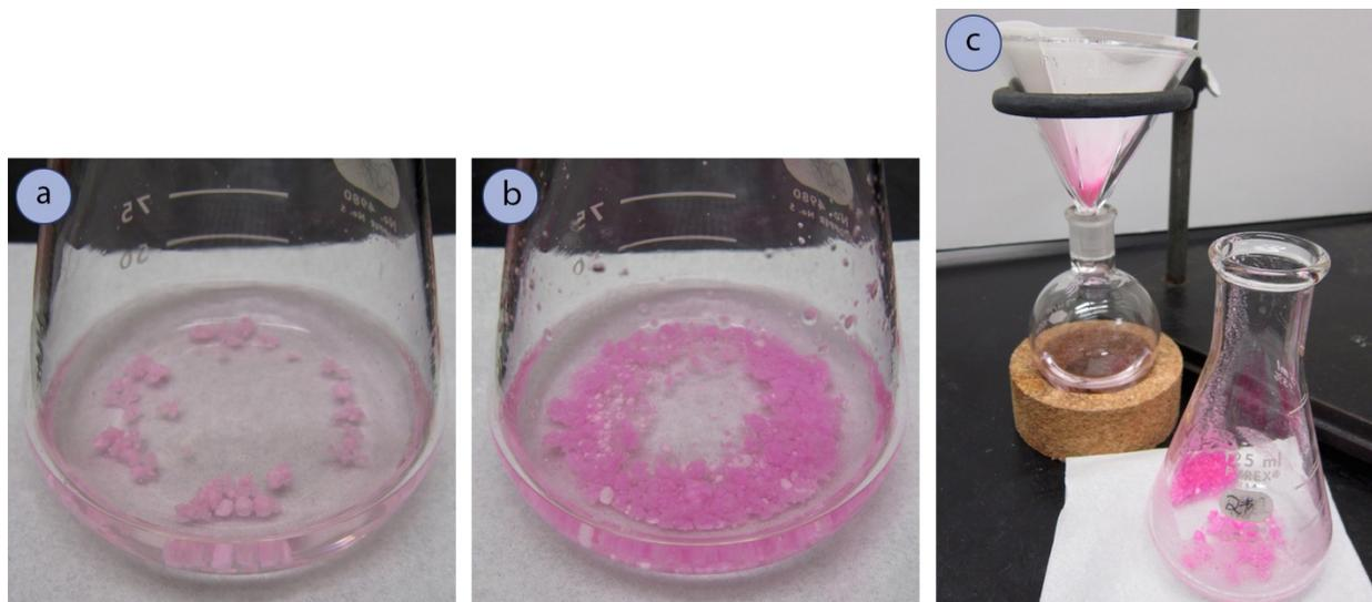
**Figure 4.45:** a) Ethyl acetate layer with a small amount of dissolved red food dye. With addition of white anhydrous  $\text{MgSO}_4$ , the drying agent turned pink, showing that the drying agent has adsorbed the dye, b) With more  $\text{MgSO}_4$ , the drying agent became pinker, c) Even after a rinsing step, the drying agent retained its pink color.
