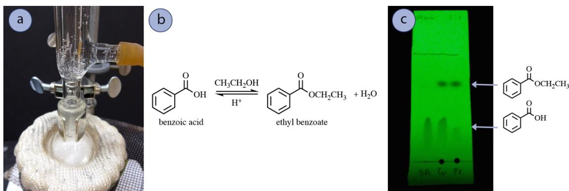
**Figure 4.56:** a) Refluxing reagents, b) Reaction scheme, c) TLC after 1 hour reflux, where the first lane (BA) is benzoic acid, the second lane (Co) is the co-spot and the third lane (Pr) is the reaction mixture (ran with 1:1 hexanes:ethyl acetate and visualized with UV light).
