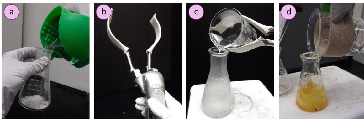
**Figure 1.26:** Pouring liquid with a) hot hand protector, b+c) Beaker tongs, d) paper towel holder.
