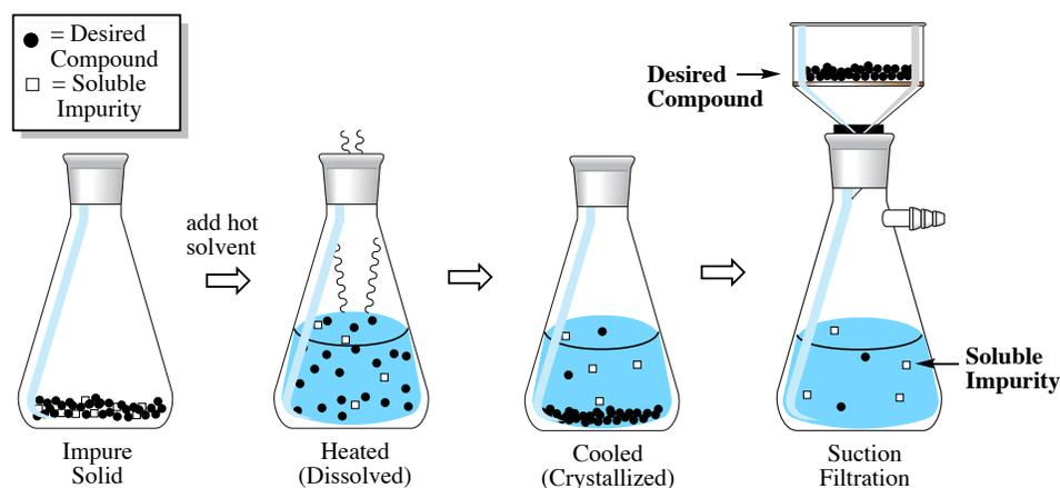
Figure 3.27: Crystallization Sequence to remove a soluble impurity.
