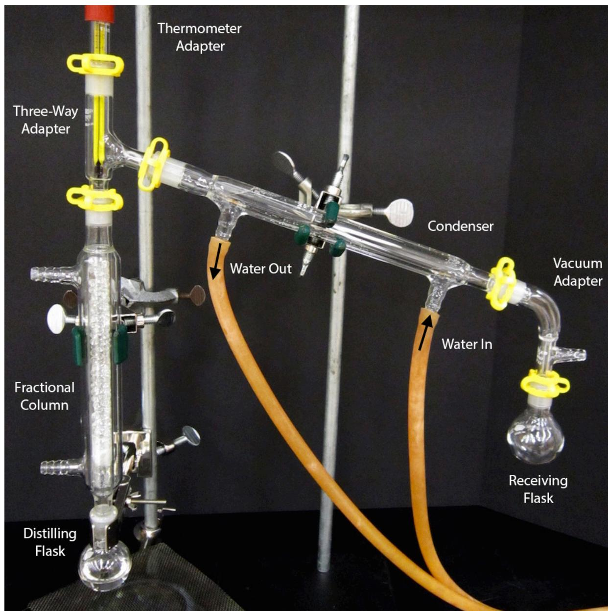
Figure 5.43: Fractional distillation apparatus.
