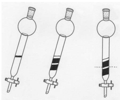
Figure 2.67: Effect of a crooked column on separation.
