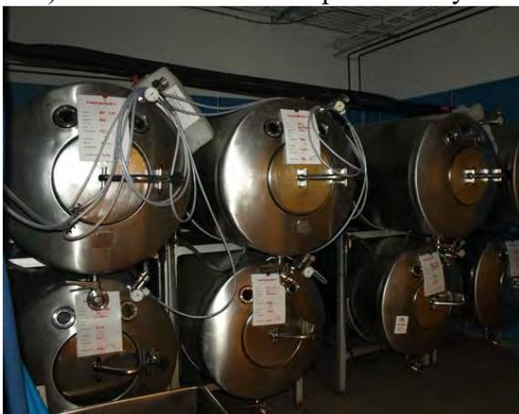
Figure 6.26 The fermentation of grape juice to make wine produces CO<sub>2</sub> as a byproduct. Fermentation tanks have valves so that pressure inside the tanks can be released. (credit: Clark et al. / [Biology 2E OpenStax](#))
