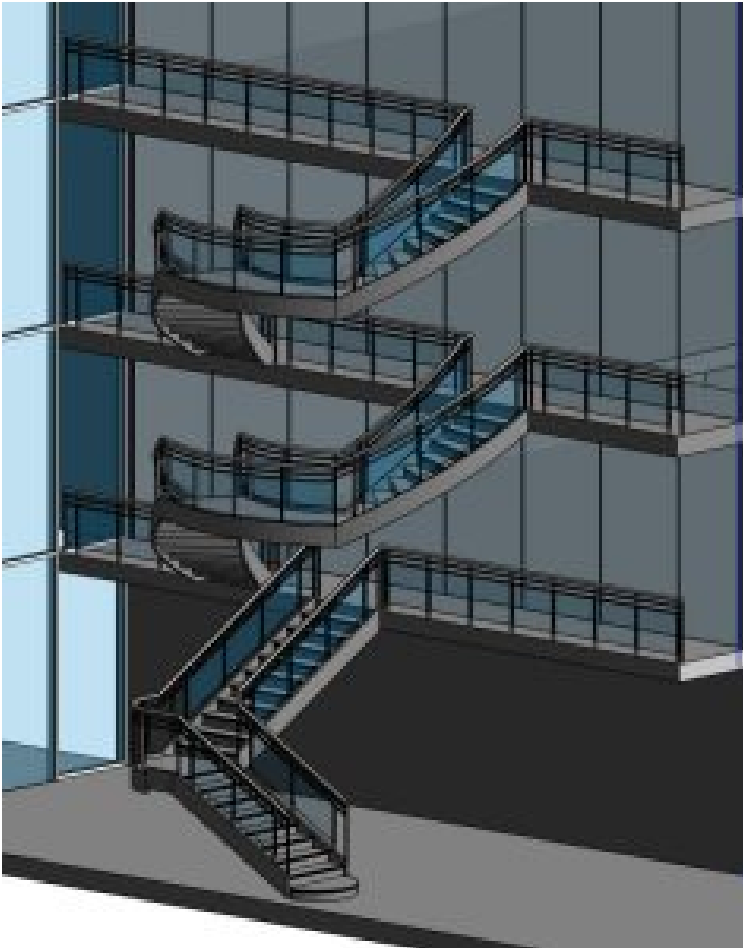
Figure 4.14 Mezzanine railing completed for Levels 2, 3, and 4 (Two walls in the 3D view are hidden to show the railings)
