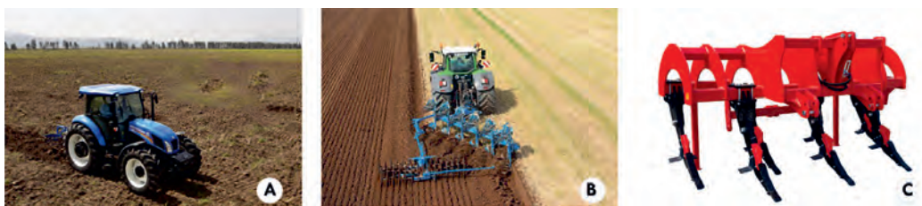
Figure 14.1. Crop cultivation equipment: A) tractor, B) plough, C) subsoiler
