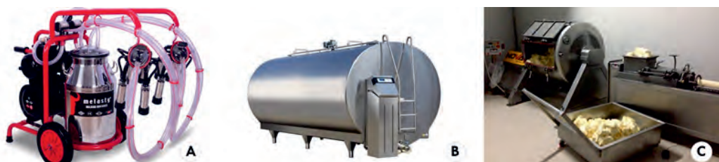
Figure 14.6. Dairy machinery: A) milking machine, B) milk cooler, C) butter churner
