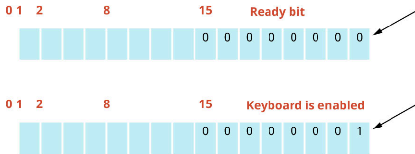
Figure 6.9 In this device register for a keyboard, the ready bit is set to 1 for when a user starts using the keyboard. (attribution: Copyright Rice University, OpenStax, under CC BY 4.0 license)
