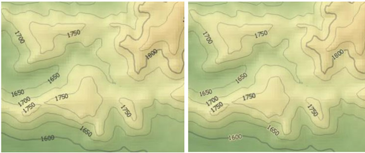
Figure 2.2.9 Simple contour labels (left); improved legibility with a subtle halo (right) Credit: Maps by Cary Anderson, Penn State Department of Geography, Data Source: The National Map.
