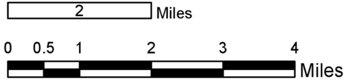
Figure 2.7.3 Two different scale bars created in ArcGIS Pro. Credit: Cary Anderson, Penn State University.
