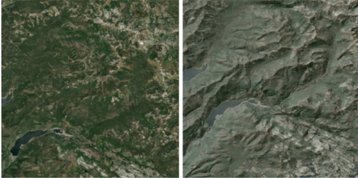
Figure 1.6.4 An aerial image from California (left), an aerial image with a transparent hillshade from a similar location (right) Credit: Cary Anderson, Penn State University, Data Source: The National Map
