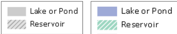
Figure 1.7.3 Categories of waterbody features using pattern (left), and pattern and hue (right) Credit: Cary Anderson, Penn State University.
