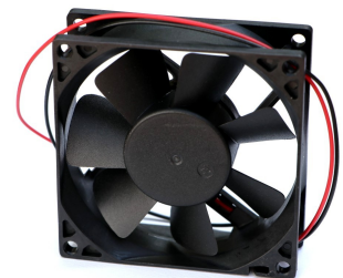
Figure 7.25 A small boxer fan for cooling electronic components.
