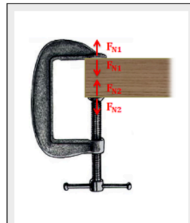
If we ignore the weight of the two objects, this clamp will also have two pairs of Third Law forces. The first will be a set of normal forces at the top point of contact (one force on the wood and one force on the clamp) and the second will be another set of normal forces at the bottom point of contact (one force on the wood and one force on the clamp). Image adapted from Public Domain image, no author listed.
