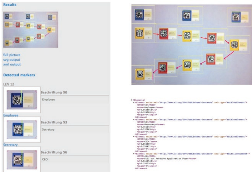
Fig. 7.9 Card-model recognition for conceptual representation: web-interface (left), recognition results (top right), XML-based model representation (bottom right) (released under a Creative Commons Attribution 4.0 International License (CC BY 4.0))
