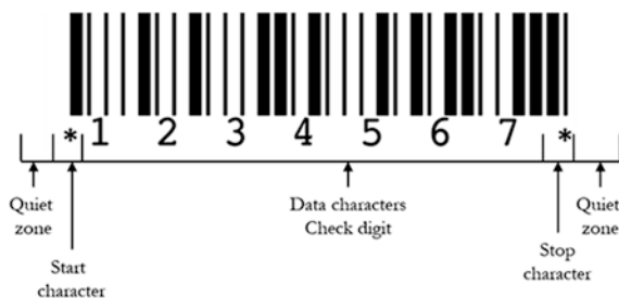
Fig. 6.1 Bar code structure (Source Adapted from Zsifkovits 2013)
