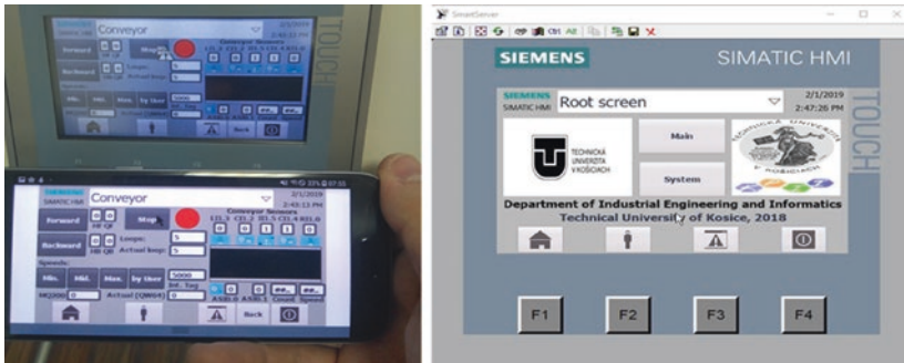
Fig. 11.18 Remote monitoring of inspection device by mobile phone (left) and by PC (right)
