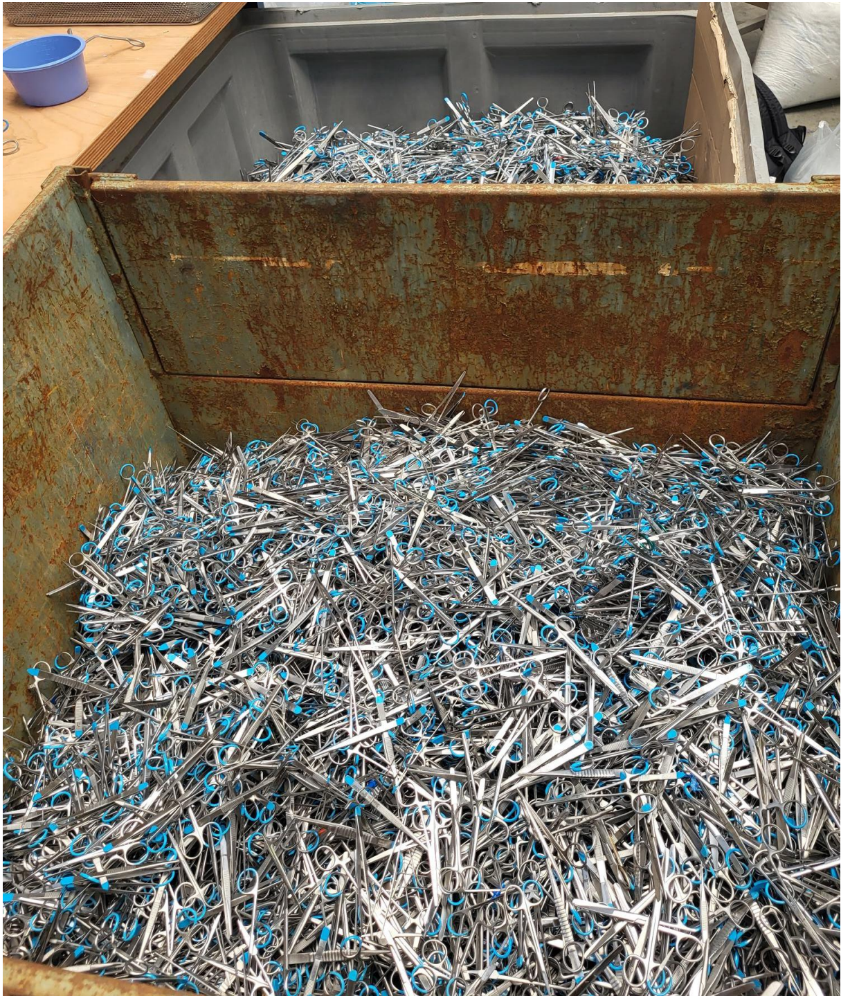
Figure 1. Collected stainless steel (SS) disposable instruments. These instruments are typically made in Pakistan and shipped throughout the world to be used once, after which they are disposed of and often incinerated. This type of stainless steel is generally SS304. Photo by Bart van Straten.
