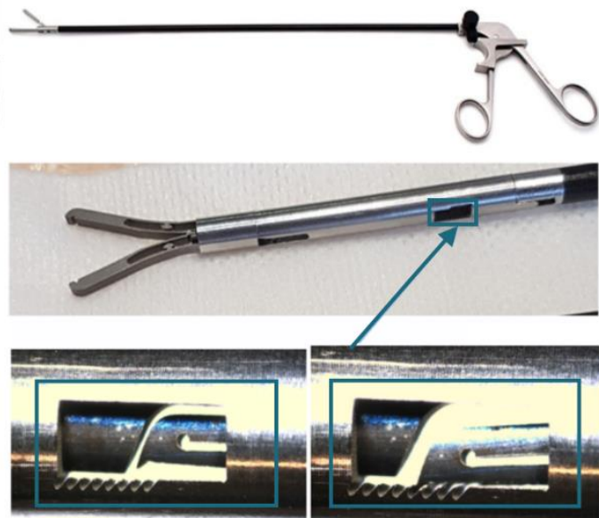
Figure 7. Top: A force-limiting shaft (green box) that expands when overloaded and thus prevents damage to tissue. Below: Pulling on the rod results in a movement and mechanical lock of the flexing element. Photo by Tim Horeman.
