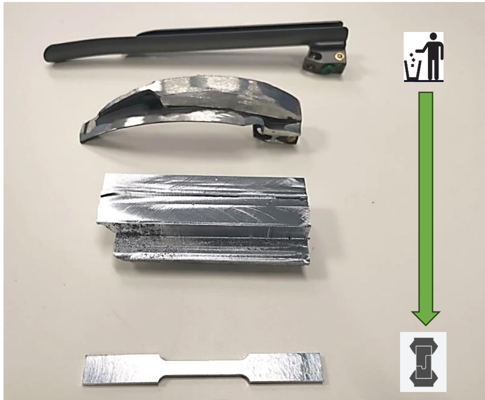
Figure 5. The material transformation steps from collected Zamak instruments (top) that are cast into blocks (middle) before being turned into dog bones (below) for tensile testing. Photo by Bart van Straten.
