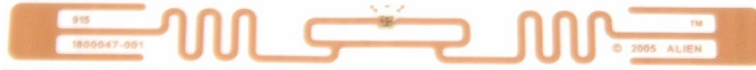
Figure B.2: A tag used in a 900 MHz-band passive RFID system. This tag is about 10\text{ cm} \times 1\text{ cm} . The IC is the small rectangular device located near the center of the tag. The antenna is essentially a resonant dipole which has been compressed in length using a combination of “meandering” and end loading. Trademark and ©ALIEN. Used under fair use.
