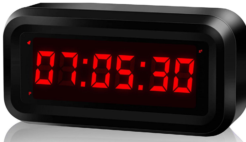
Figure 3.16. Offering second level precision when setting a wake-up alarm comes with a cost: added complexity and more room for error, when setting the alarm time, just to cover an admittedly marginal scenario.
