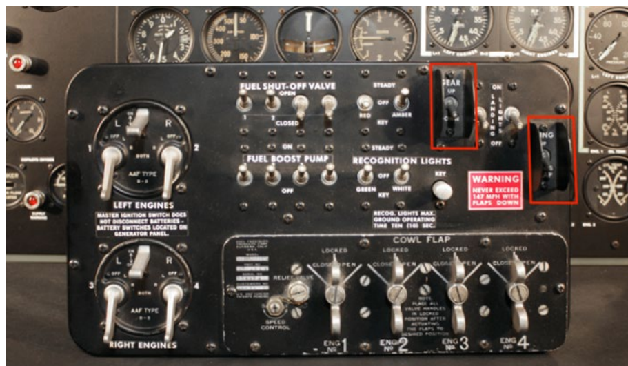
Figure 1.2. The two toggles, one for the landing gear and the other to control the wing flaps.
