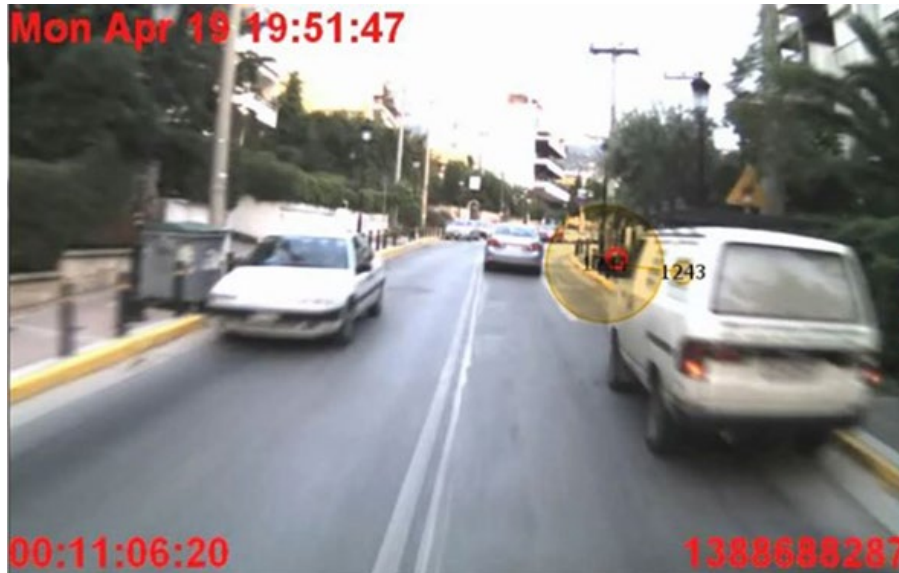
Figure 4.3. A frame of the eye tracking study, showing the focusing of the motorcyclist on a side view mirror to understand the intentions of the driver.
