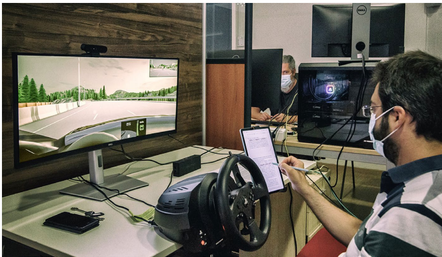
Figure 7.22. A user testing setup situated in a dedicated usability lab. A participant engages in a secondary task in automated driving mode on a driving simulator.
