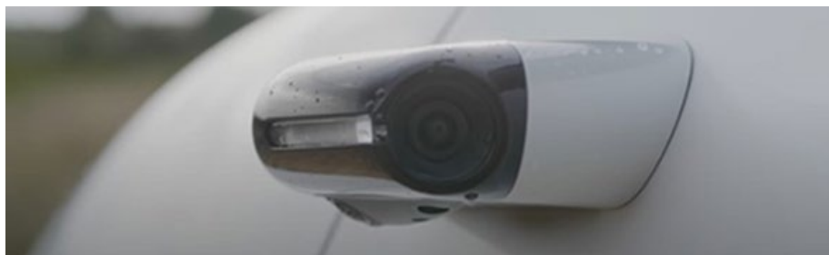
Figure 4.2. A camera replacing the side view mirror on a car.
