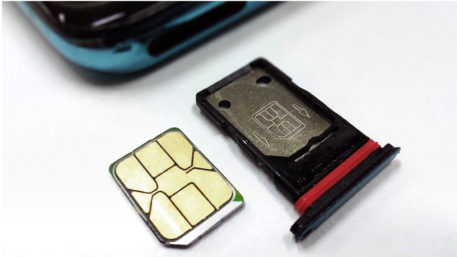
Figure 3.11. The cut-out of the SIM card is purposefully designed as a physical constrain to prevent erroneous placement of the card in an electronic device.
