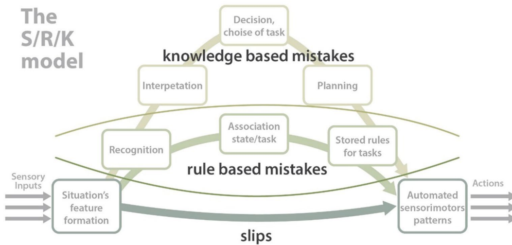
Figure 3.18 The attribution of slips and mistakes in the SRK model.
