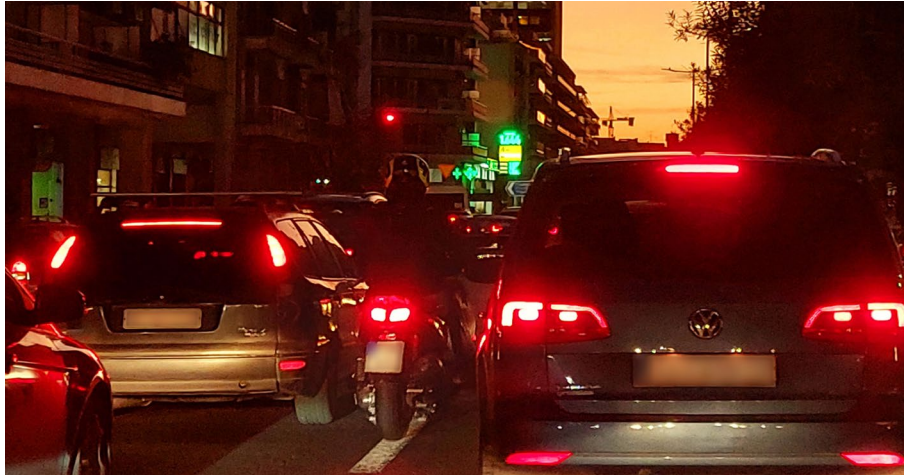
Figure 1.4. The third brake light, mounted in the rear windshield, became mandatory in cars after similar studies.
