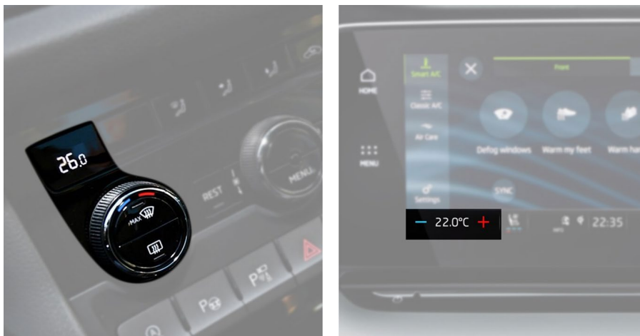
Figure 8.30. Two alternative controls for cabin temperature in a car, a physical knob (left) and touchscreen buttons (right)
