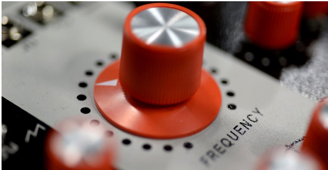
Figure 3.20. Failing to set this knob to the exact desired value, due to the tight configuration of possible states, is considered a slip. In this case, the intended action is probably correct, but the user fails in terms of the dexterity needed. Instead, if the user wanted to adjust the volume but decided to turn the frequency knob instead, then, this is considered as a mistake. At the same time, if the knob provides no tactile feedback when switching between states, this may lead to omission errors.
