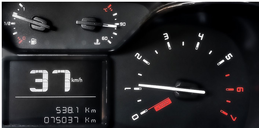
Figure 8.33. A digital alphanumeric speedometer, next to an analog rpm gauge. Alphanumeric values are best suited for observing speed limits while analog readings are best suited for rpm range monitoring.
