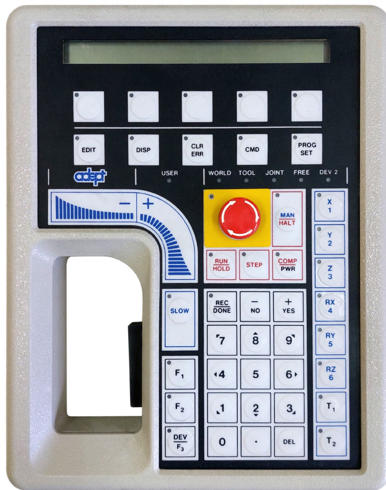
Figure 8.29. A manual robot controller teach pendant. The emergency stop button is readily detectable through its position, size and color. What is more, to prevent its accidental effectuation a rotating action is required instead of a pushing action.
