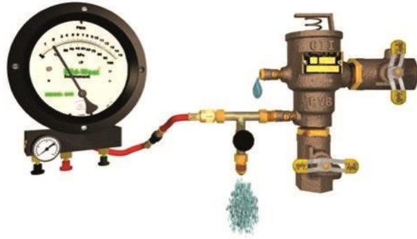
Figure 8-14—Using a bleed valve arrangement
