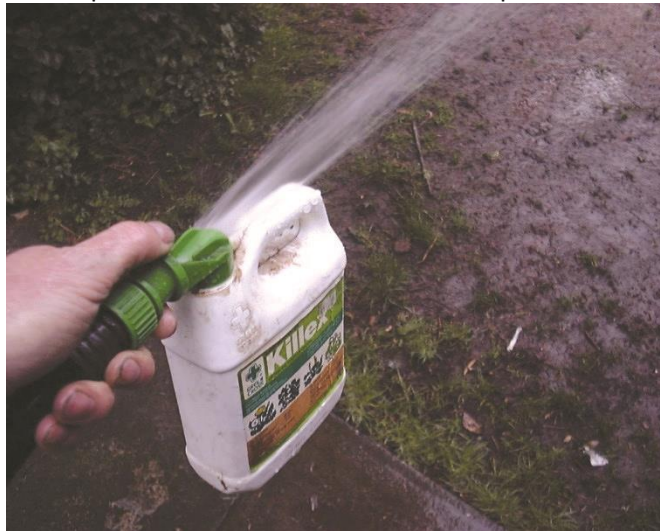
Picture of weed sprayer using venture effect to draw weed killer into the high velocity water flow.
