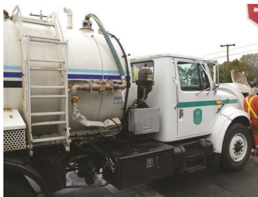
Figure 6-75—Picture showing truck mounted RP and AG at filler
