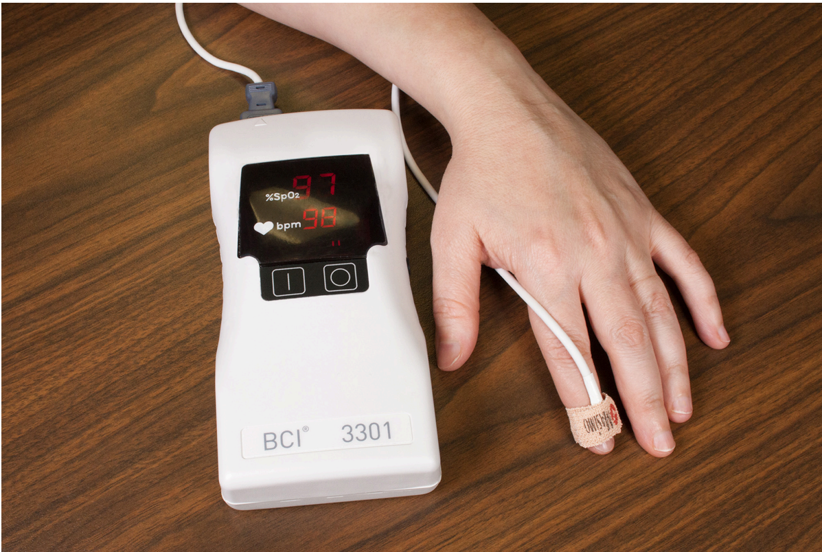
Figure 4.2: Pulse oximeter with sensor taped around finger.
