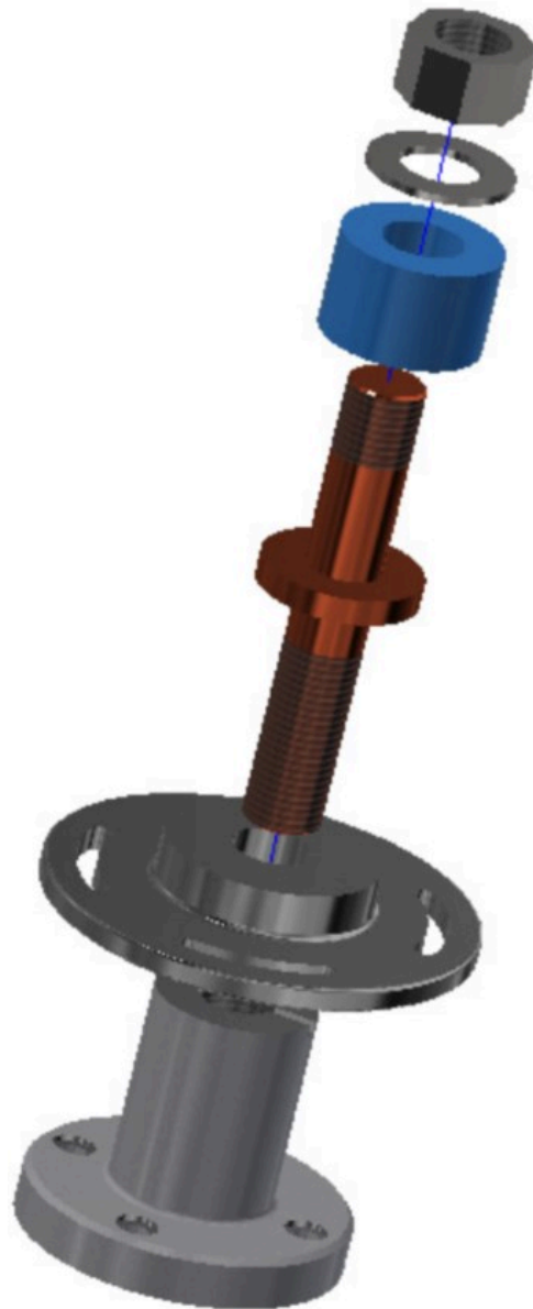
Figure 23-1 An Exploded and Rotated Presentation Model
