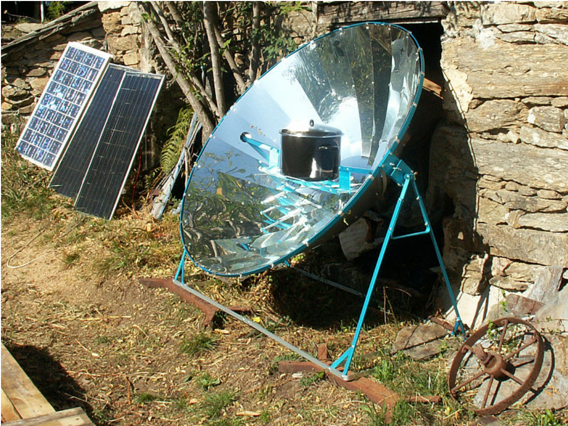
Figure 8.63: Solar Cooker. Photograph shows solar heating system. Source: Atlascuisinesolaire via Wikimedia Commons 181 .
