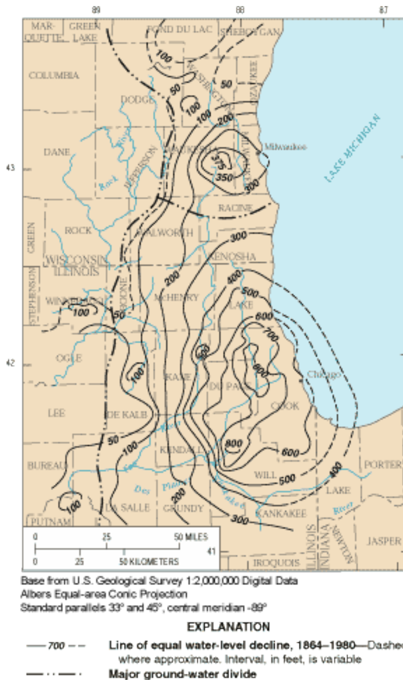
Figure 5.20: Drop in Water Table in a Confined Aquifer in the Area of Chicago, Illinois and Milwaukee, Wisconsin, U.S. from 1864 - 1980 Source: United States Geological Survey 23
