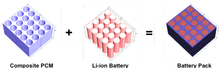
Figure 8.65: Application with PCM Technology. A pack of Li-ion batteries kept at a narrow temperature range with a proper use of passive thermal management system. Source: AllCell's PCM Technology©
