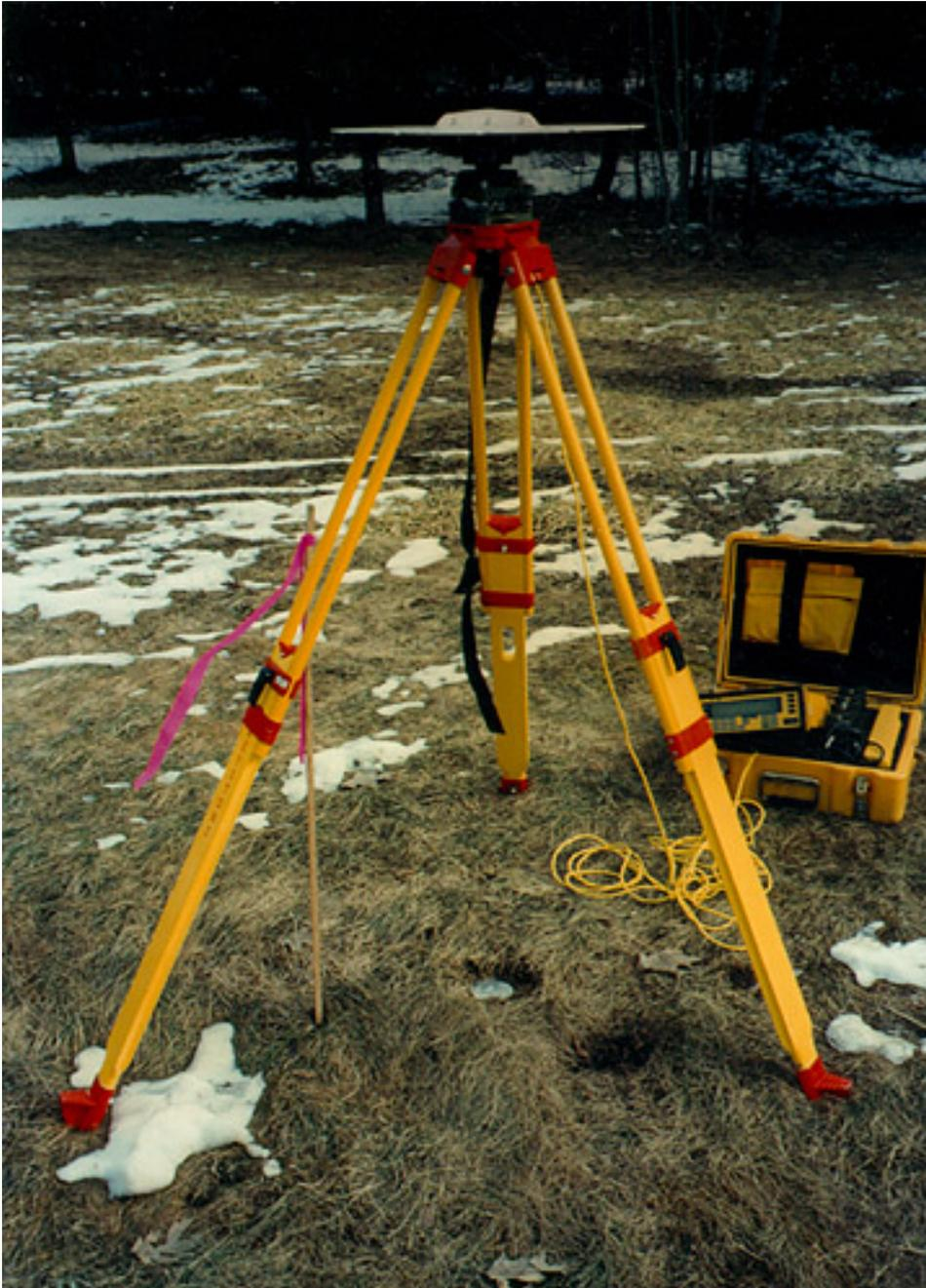
GPS base station used for differential correction. Notice that the antenna is located directly above a control point monument.
