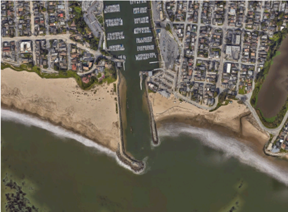
Figure 13.5.2 The jetties protecting Santa Cruz harbor, California. Sand has accumulated on the left (north) side of the harbor, and the beach is eroded on the right (south) side (Google Maps, Map Data: Google).
