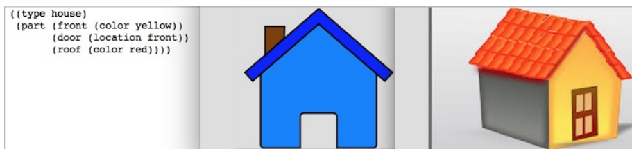
Figure 17.3: Right: 3D, real-world house; Middle: 2D model of 3D real-world house; Left: computer representation of 2D model
