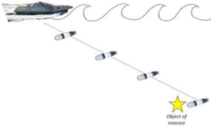
Figure 6.5: Depiction of an Undersea Communication Bridge
