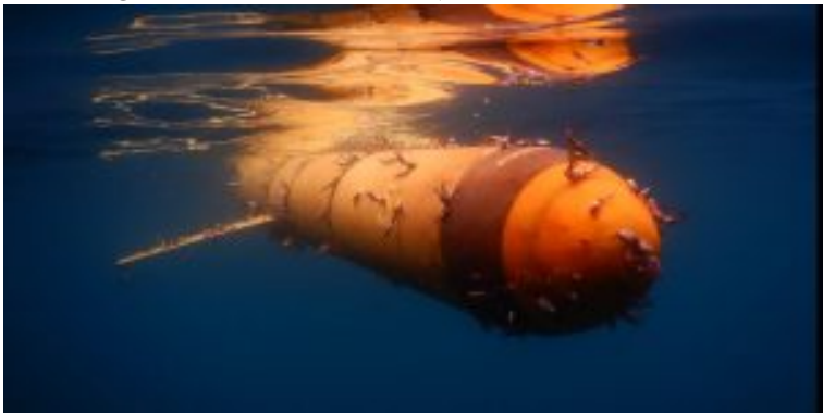
Figure 3.17 Teledyne Marine's Slocum G2 Glider autonomous underwater vehicle (AUV)
