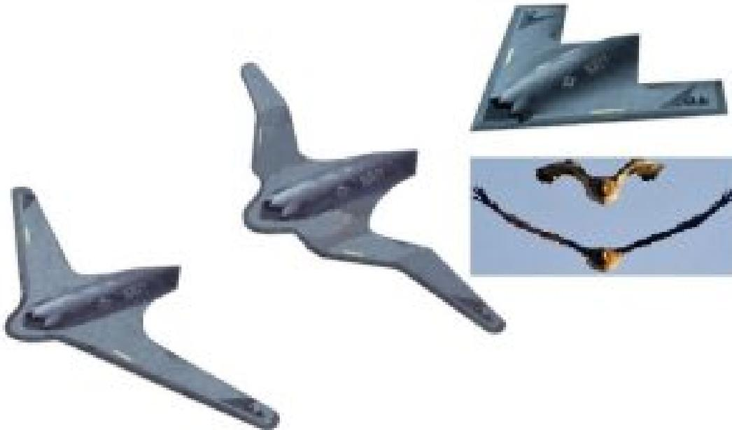
*Note:* Different morphing configurations can provide the ultimate configuration relative to the action performed. The above image has standard flight, Lottering, and dash configurations.
