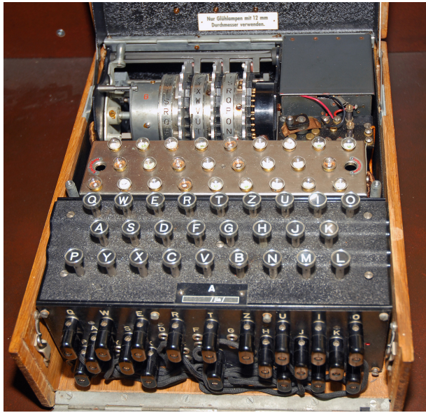
Fig. 1. Three wheel Enigma machine
