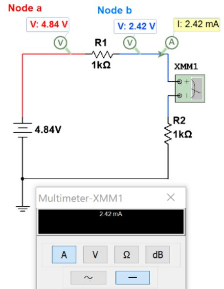
**Figure 1.8:** Circuit showing current measured with a Multimeter.
