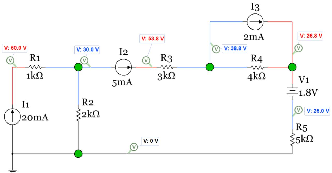
Figure 1.11: Circuit for Example 1.11
