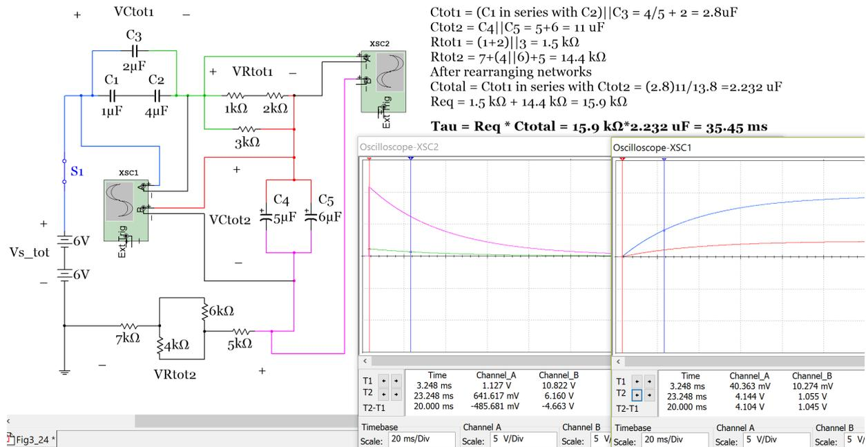
Figure 3.24b: Circuit for Example 3.8 and oscilloscope plots.
