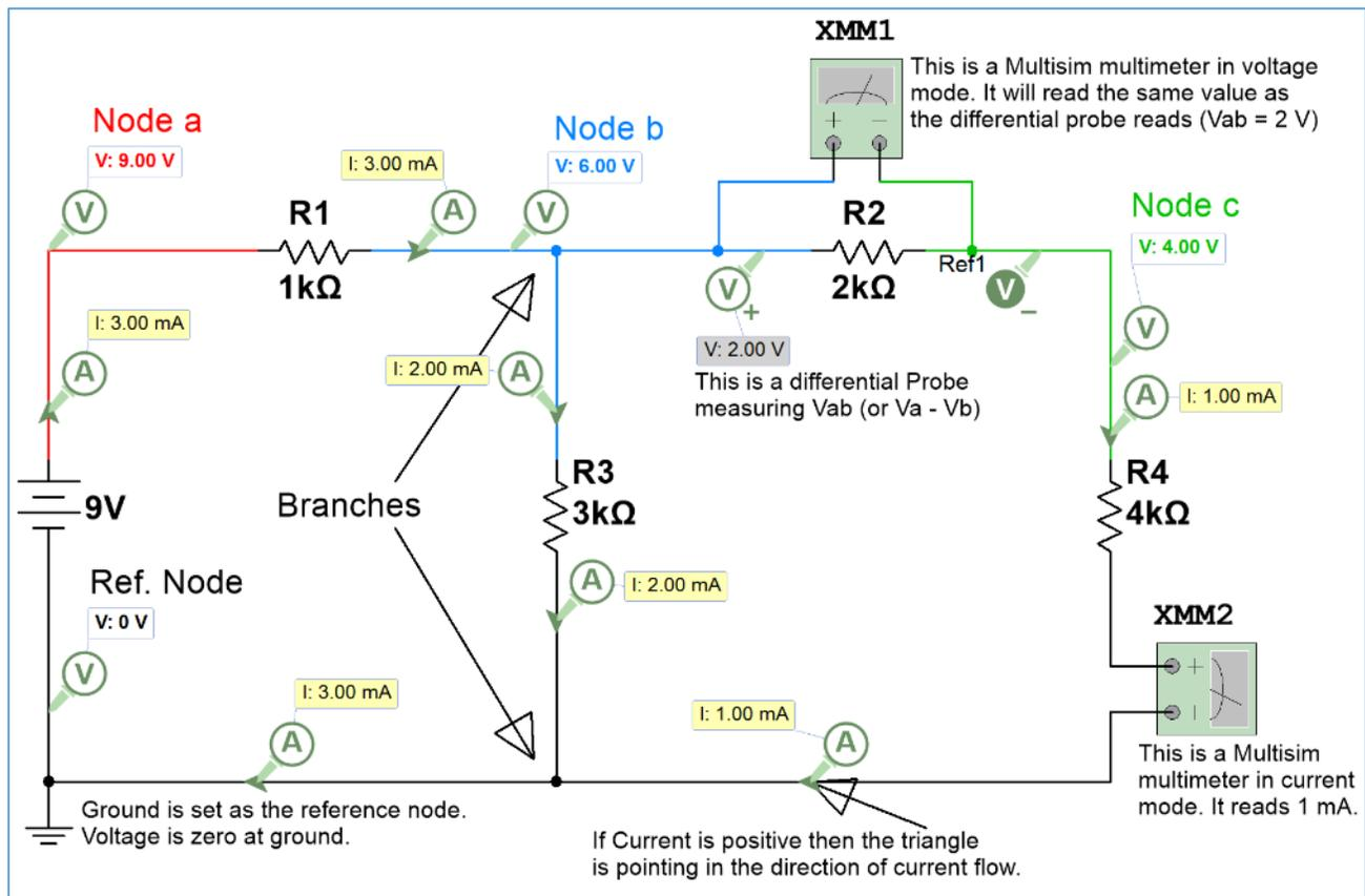
**Figure 1.7: Circuit showing probes, Multimeters, branches, and nodes.**
