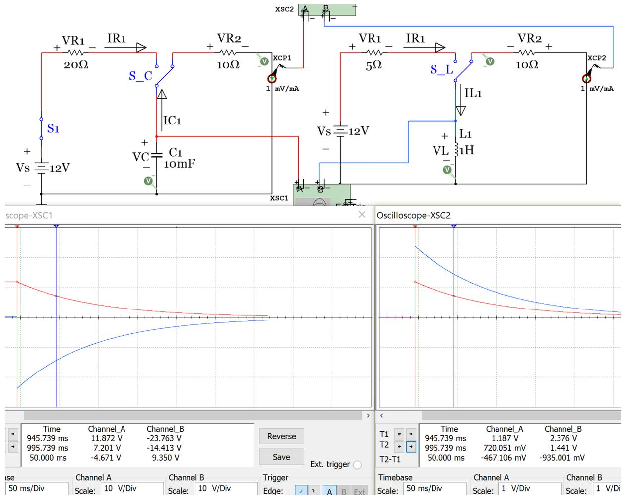
Figure 3.25: RC and RL discharging circuits for Example 3.9.
