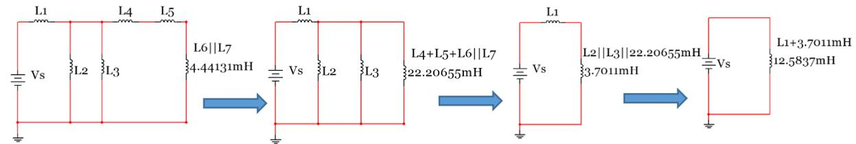
**Figure 3.12: Combining inductors for example 3.2.**
