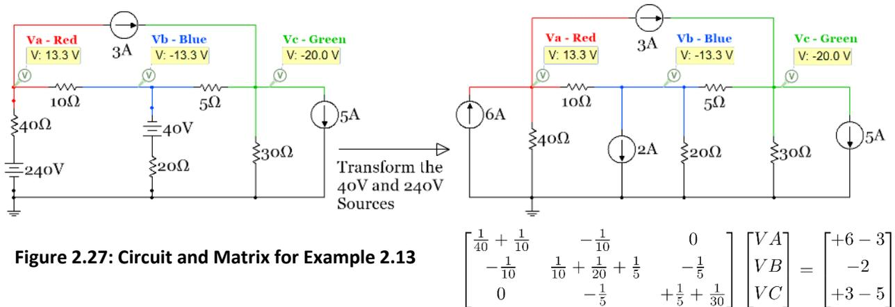
**Figure 2.27: Circuit and Matrix for Example 2.13**
