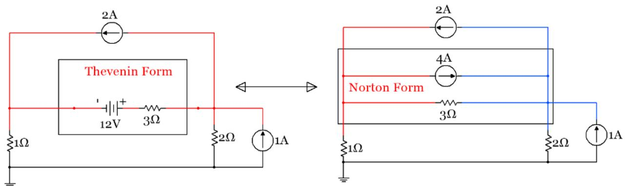
**Figure 2.5: Circuit for Example 2.2**
