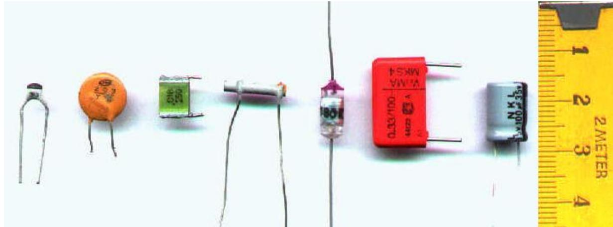
Figure 3.2: Different types of capacitors. From left: multilayer ceramic (MLCC), ceramic disc (see [Figure 3.3a](#)), multilayer polyester film, tubular ceramic, polystyrene, metalized polyester film, aluminum electrolytic. [Photo © aka and used under a CC BY-SA 3.0 license.](#)
