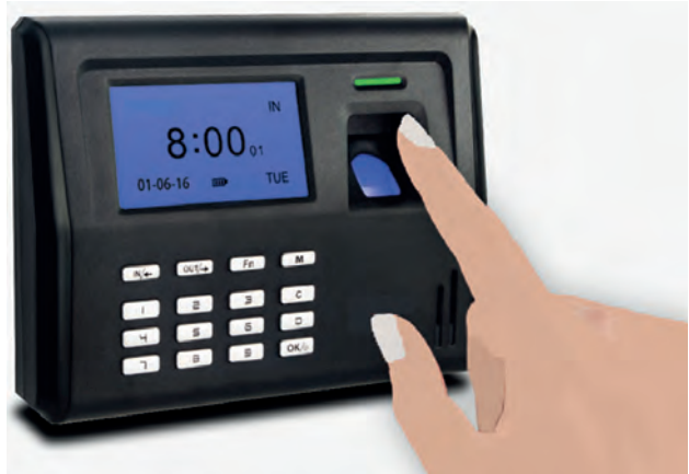
Figure 1.18: Digital Identity Attendance controlling device using fingerprint
