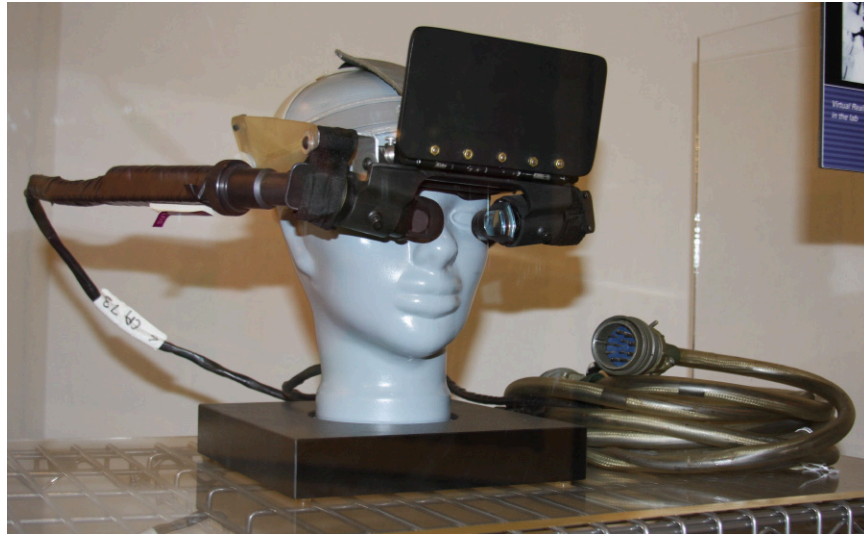
Figure 10.2 Known as the “Sword of Damocles,” Ivan Sutherland and his research team created this first head-mounted virtual reality device in 1968. (credit: modification of work “Virtual Reality Headset Prototype” by “Pargon”/Flickr, CC BY 2.0)
