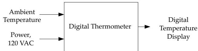
Figure 5.9: Level 0 digital thermometer functionality.
