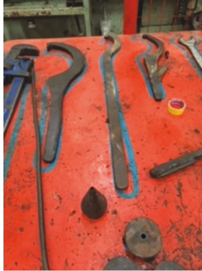
Fig. 1.3 Tools and their designated storage spaces in an electric cable factory in Dar es Salaam, Tanzania, 2016. (Source: Created by the author)
