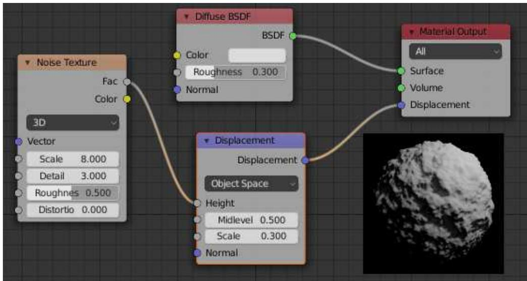
For displacement mapping to work, the surface must be finely subdivided. For the icosphere in the example, I used 4 subdivisions when I created it, and then I added a Subdivision Surface modifier with three levels of subdivision to divide it even more finely.
