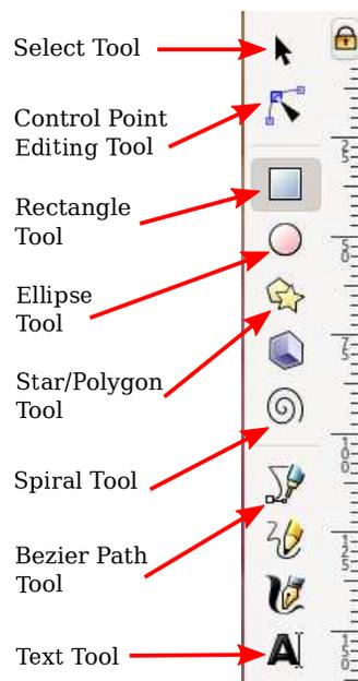
You can also get a description of a tool by hovering your mouse over its icon. (The same is true for most interface elements.) It’s a good idea to learn some of the keyboard equivalents, such as F1 or S for the select tool.
