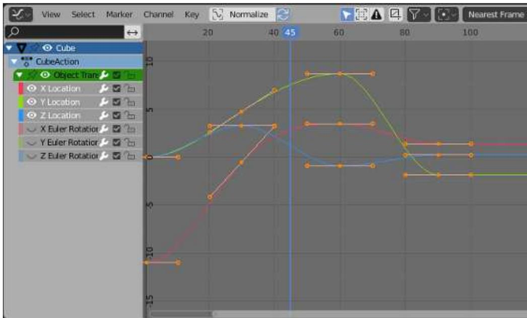
Each curve controls one animated property, plotting the value of the property on the vertical axis against the frame number on the horizontal axis. The curves are Bezier curves by default. In the picture, the Rotation curves have been hidden (by clicking the “eyes” next to the curve names), and the three visible curves and all their Bezier handles have been selected (by hitting the “A” key while the mouse is over the graphs).
