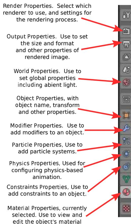
In this picture, the Materials button has been clicked. With the materials button selected, the rest of the editor panel, to the right of the buttons, is filled with controls for setting the material properties of the selected object. Most of the controls don’t appear until a material has been
