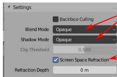
In the **Material Properties** for the object, under “Settings,” turn on “Screen Space Refraction”. You might need to increase “Refraction Depth” to a value greater than zero.
