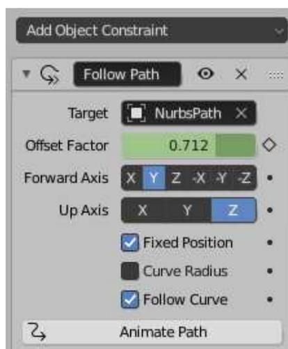
You will need to use the “Target” menu to select the name of the curve that you want the object to follow. To get the object to actually jump onto the curve, you will need to clear its Location, not its Origin. (Select the object and use ALT-G, or use the “Location” command in the “Clear” submenu of the “Object” menu.)
