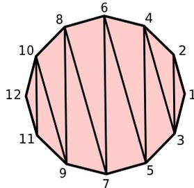
A disk can be approximated by a polygon, and a polygon can be rendered in WebGPU as a primitive with topology "triangle-strip."
